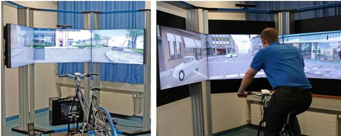
Figure 6.1: Three-display setup of the FIVIS bicycle simulator including bicycle input at the Institute of Visual Computing of Hochschule Bonn-Rhein-Sieg in Sankt Augustin\*
