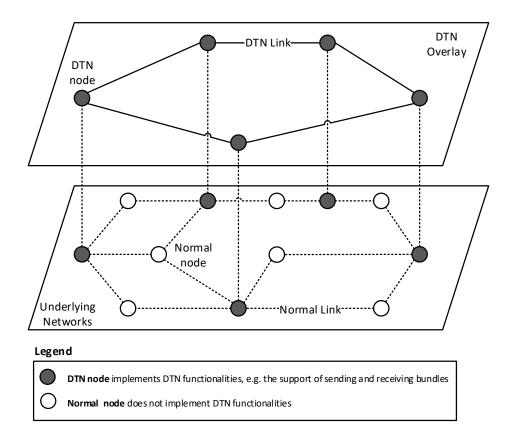
FIGURE 2.2 – DTN overlay network model
