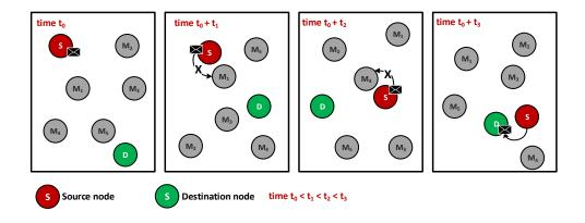
FIGURE 3.12 – Direct Delivery routing protocol sequence.
