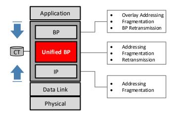
**FIGURE 6.1** – BP unified layer, integrating functionality of TCP/IP and Bundle Protocol.
