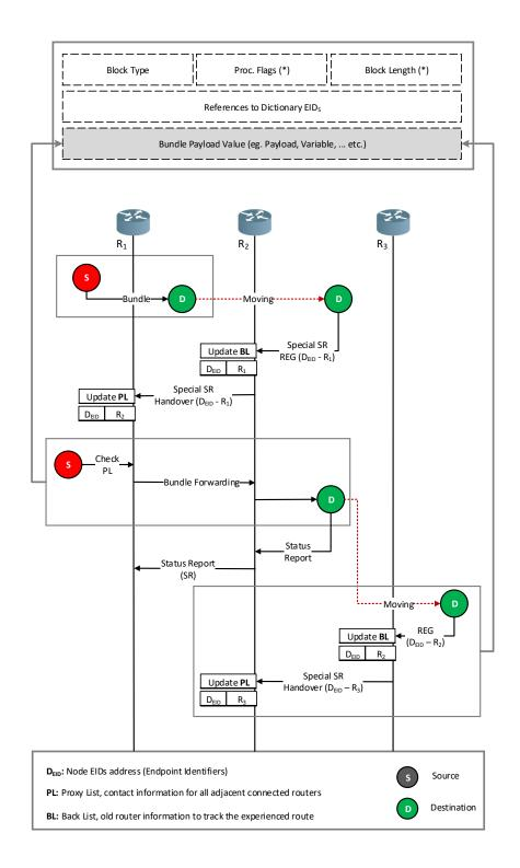
FIGURE 4.7 – Routing procedure includes handover between different regions.
