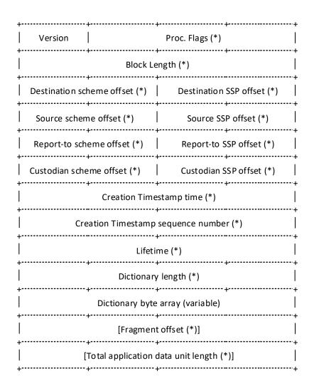
FIGURE 2.10 – The structure of Primary Bundle Block of a DTN-bundle.
