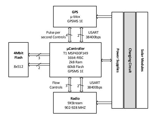
FIGURE 2.15 – Conceptual diagram of a ZebraNet node [111].
