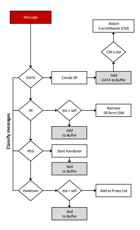
FIGURE 4.5 – A block diagram of messages classification and actions.
