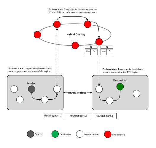
FIGURE 4.1 – HIDTN protocol states in hybrid DTN routing.
