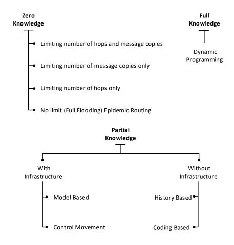
FIGURE 3.4 – Combination of the various DTN routing protocols classifications.
