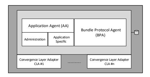
FIGURE 2.9 – A graphical representation of a Bundle node.
