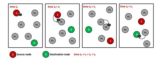
FIGURE 3.13 – First Contact routing protocol sequence.
