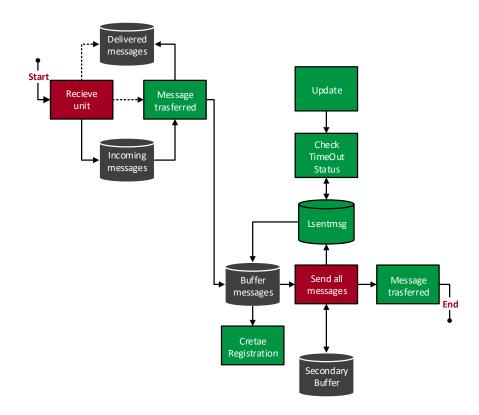
FIGURE 5.1 – Functional block diagram of routing algorithm implementation.
