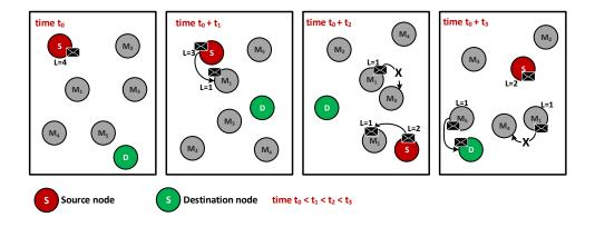
FIGURE 3.9 – SnW: Source Spray and wait routing protocol sequence.
