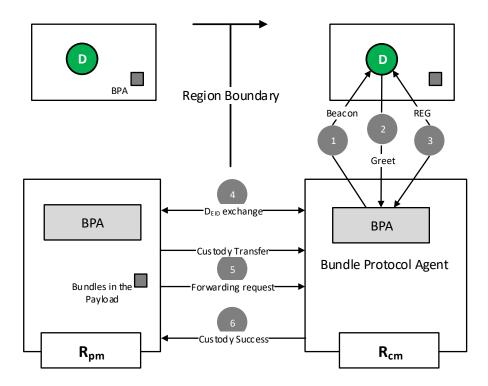
FIGURE 4.6 – Control message exchanges.
