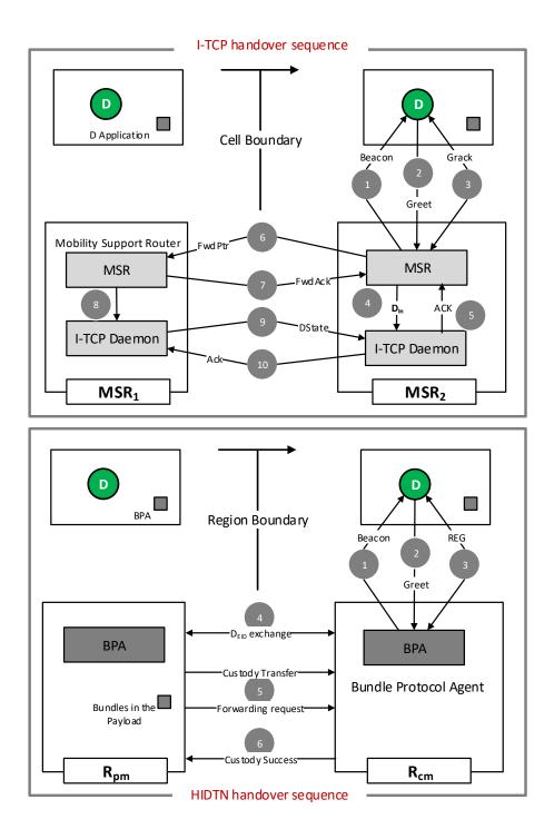
**FIGURE A.1** – *HIDTN vs. I-TCP* - *Control message exchange between routers and end-nodes during handover.*
