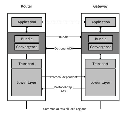
FIGURE 2.8 – Internal architecture of the Bundle Layer.
