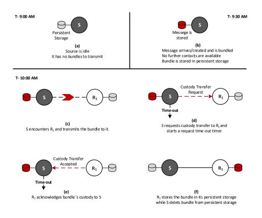
FIGURE 2.5 – Example: How the mechanism of custody works.
