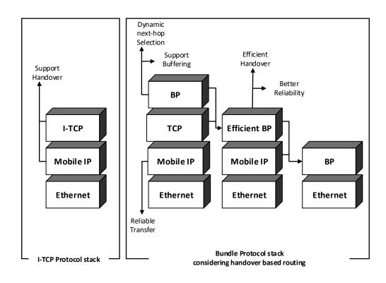
FIGURE A.2 – Protocol Stack of I-TCP and Bundle Protocol.
