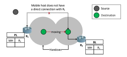
FIGURE 4.8 – Registration procedure after moving between different regions.
