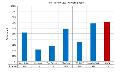
FIGURE 5.4 – Delivery ratio without infrastructure - all mobile nodes.
