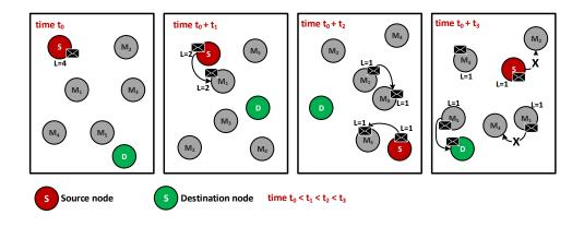
FIGURE 3.10 – SnW: Binary Spray and wait routing protocol sequence.
