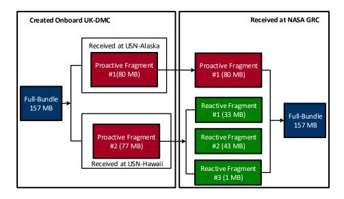
FIGURE 2.13 – Large File Transfers using Proactive and Reactive DTN [102].
