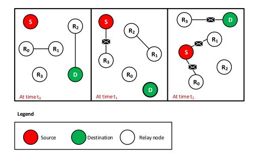
FIGURE 3.2 – Various snapshots a time-evolving Delay Tolerant Network.
