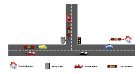
FIGURE 2.14 – Interactions between nodes in VDTN networks.
