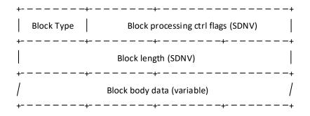
FIGURE 2.12 – The structure of Bundle Extension Block.
