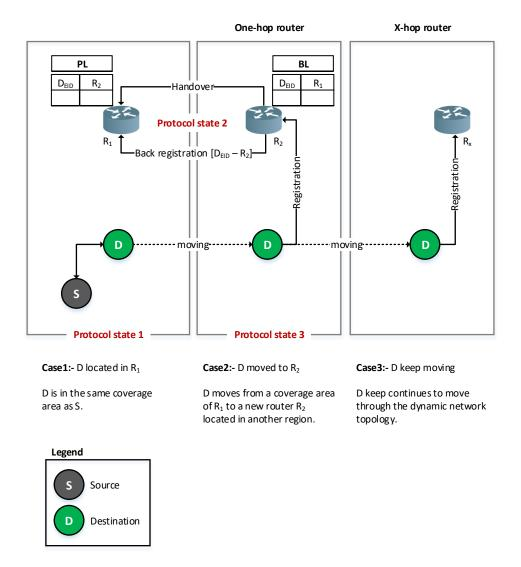
**FIGURE 4.3** – *Relay infrastructure in a hybrid DTN network to support inter-domain communications.*
