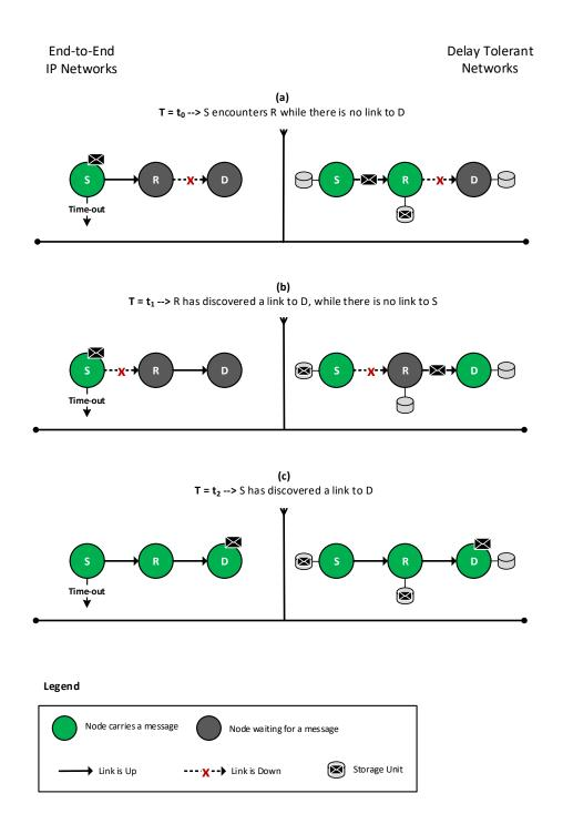
**FIGURE 2.1** – Traditional IP routing vs. DTN from the perspective of the custody transfer mechanism in different time stamps.
