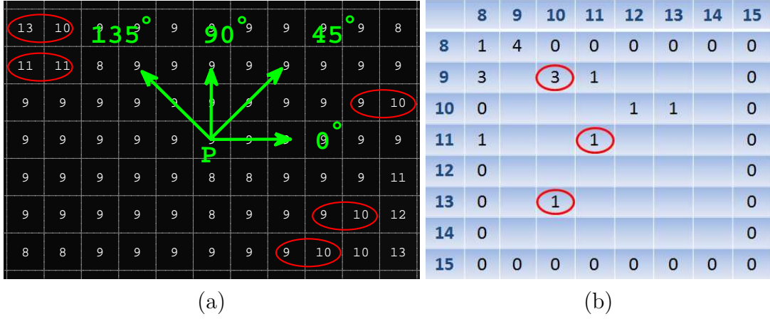
Figure 3.4: The illustration of creating a Gray-Level Co-Occurrence Matrix. (a) A patch image describes the spatial relationships of pixels that are defined by offset (the distance from the pixel of interest P , set as 3) and four directions. (b) A part of the GLCM matrix, the elements contain the appeared times of the instances, such as (13, 10), (11, 11), and (9, 10) in the patch image (a).
