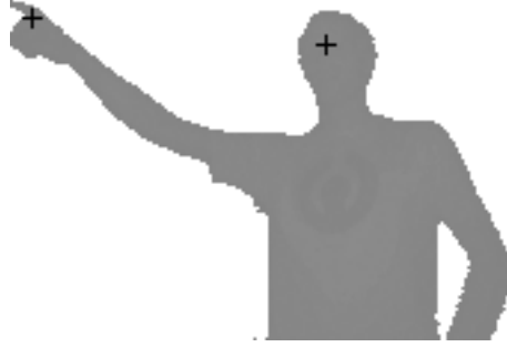
Figure 10.3: Segmented image of the user with the detected locations of the head and hand marked by crosses. The time-of-flight camera measures the three-dimensional positions of these points, which are then used to compute the pointing direction.
