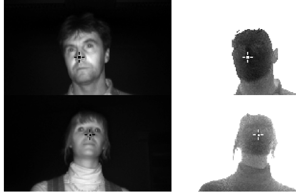
Figure 7.3: Sample images from the database of head poses. The amplitude data (left column) and the range data (right column) are given for four subjects. All pixels identified as nose pixels by our detector are marked in each image, the cross simply highlighting the locations.
