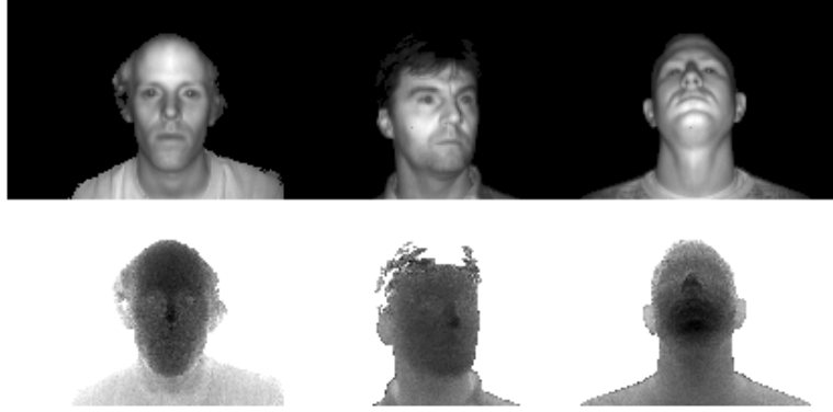
Figure 7.9: Three sample images of frontal face images taken by an SR3000 TOF camera. The top row shows the intensity and the bottom row the range data.
