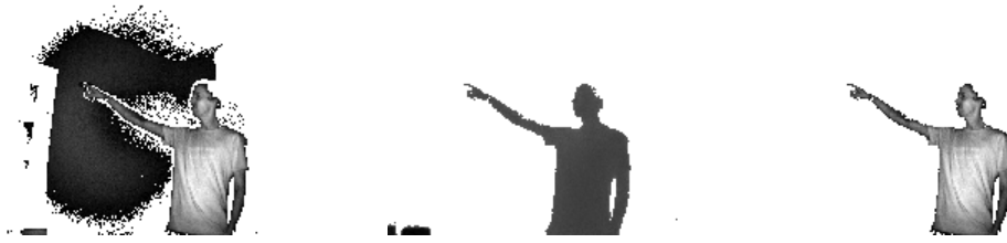
Figure 5.7: Segmentation result using combined amplitude and range data. Left: Segmented amplitude image. Center: Segmented range map. Right: Combined segmentation result. Only pixels considered foreground in both amplitude and range data are classified as foreground pixels in the final segmentation result. Furthermore, only the largest connected component of foreground pixels is retained because we are interested in the closest foreground object.
