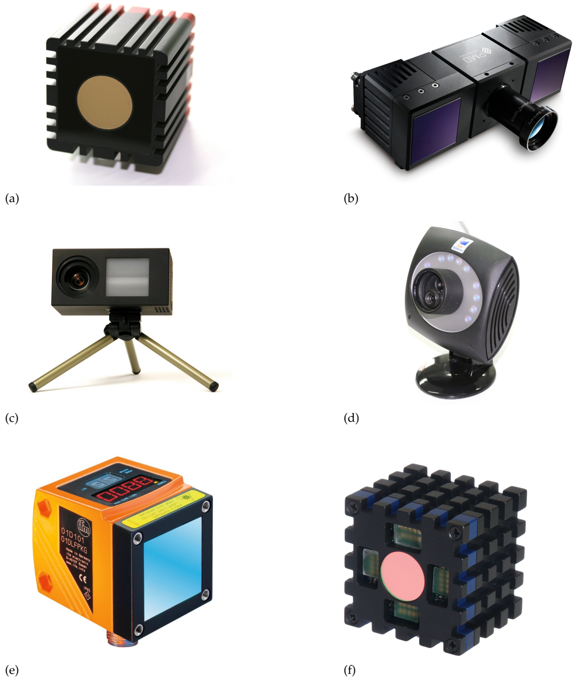
Figure 5.1: Examples of TOF cameras: (a) MESA SR4000 (image courtesy of Ingrid Brænne), (b) PMDtec CamCube (image courtesy of PMD Technologies, Siegen, Germany), (c) Canesta DP200 development platform (image courtesy of Canesta, Inc.), (d) 3DV Systems ZCam (image courtesy of Ingrid Brænne), (e) ifm electronic efector pmd (single-pixel TOF sensor, image courtesy of ifm electronic GmbH, Essen, Germany), (f) prototype camera developed by CSEM within the ARTTS project (image courtesy of CSEM SA, Neuchâtel, Switzerland).
