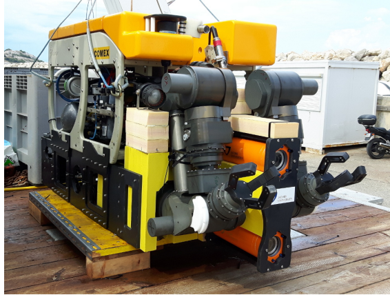
Figure 2.6 – The visual data presented in this thesis was recorded with the cameras that can be seen on the depicted ROV in the orange housing.
