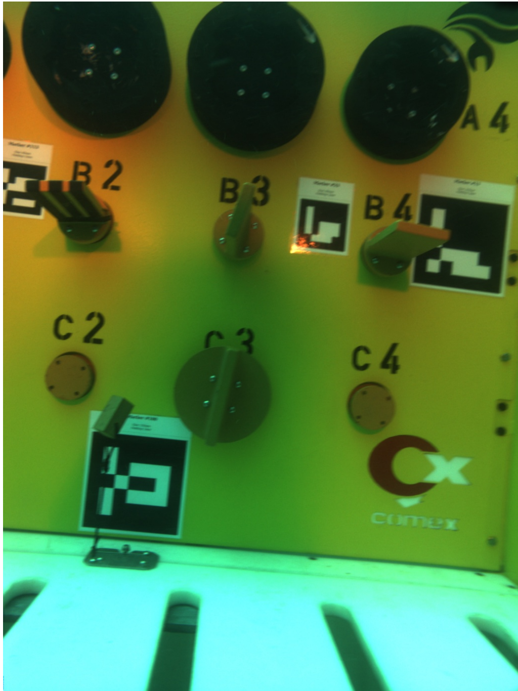
Figure 4.19 – Mock-up panel with handles that an ROV needs to operate, i.e., turn.
