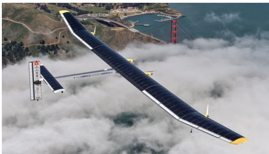
Figure 1.1: The plane Solar Impulse 2 plane is shown. The wings of the plane have 17,000 solar cells which charge batteries to also run the flight propellers overnight. The ideal flight speed is 28 mph that can double during daytime [9].
