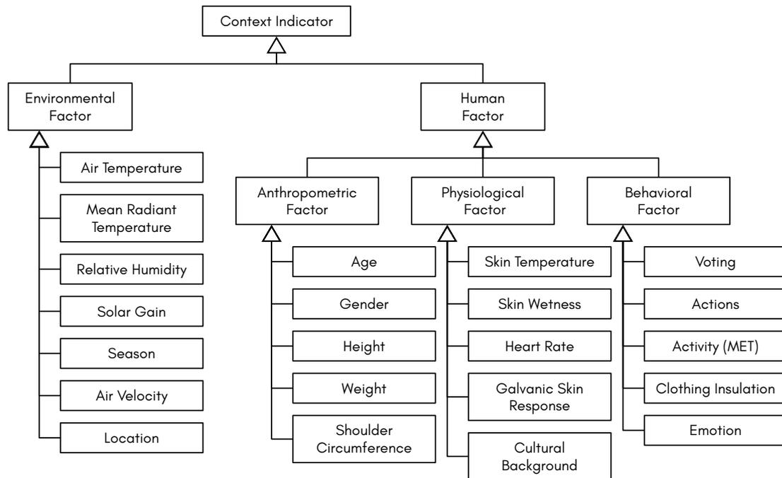
Figure 2.9: **Common Context Factors** relevant for an occupant's thermal comfort, adapted from [Fen+22] (UML Class Diagram)
