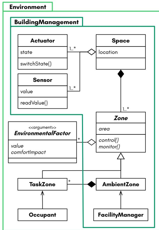
Figure 3.5: Environment Package (UML Class Diagram)
