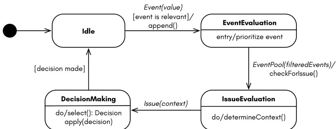
Figure 3.8: **TREATI's State Model** shows how events are transformed into issues (UML State Diagram)
