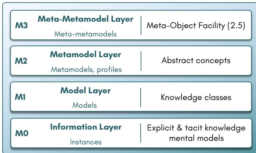
Figure 2.2: The **Meta Object Facility (MOF)** is a closed metamodeling architecture with four layers (adapted from [Obj15])
