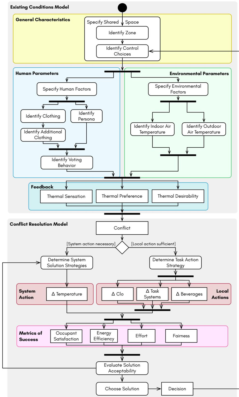
Figure 4.1: TREATI's Simulation Process (UML Activity Diagram)
