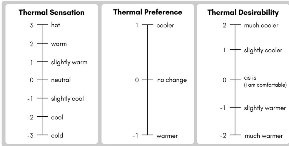
Figure 4.3: **Thermal Comfort Feedback Scales** (adapted from [FLB21; Ame19])
