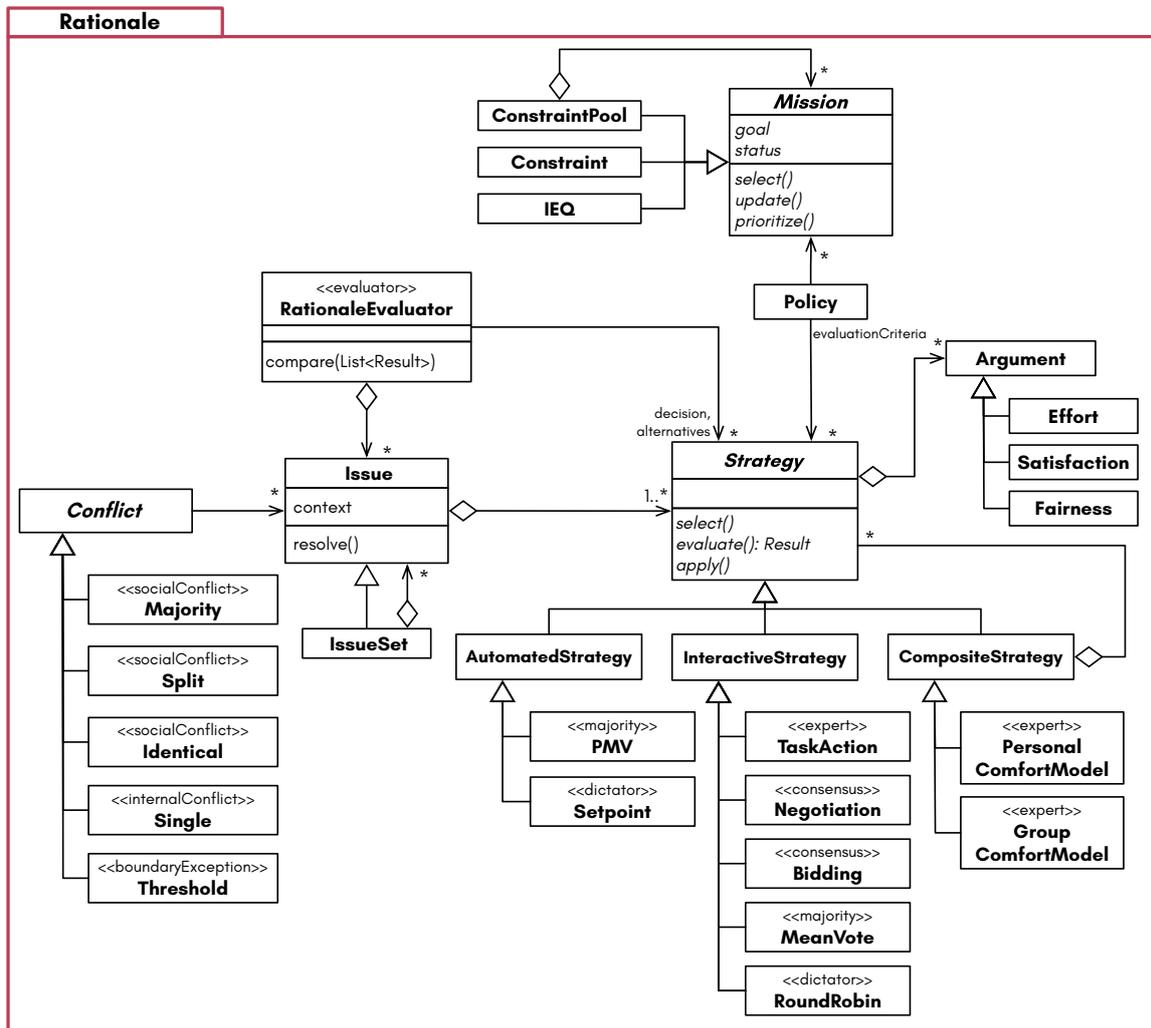
Figure 3.11: Rationale Model (UML Class Diagram)
