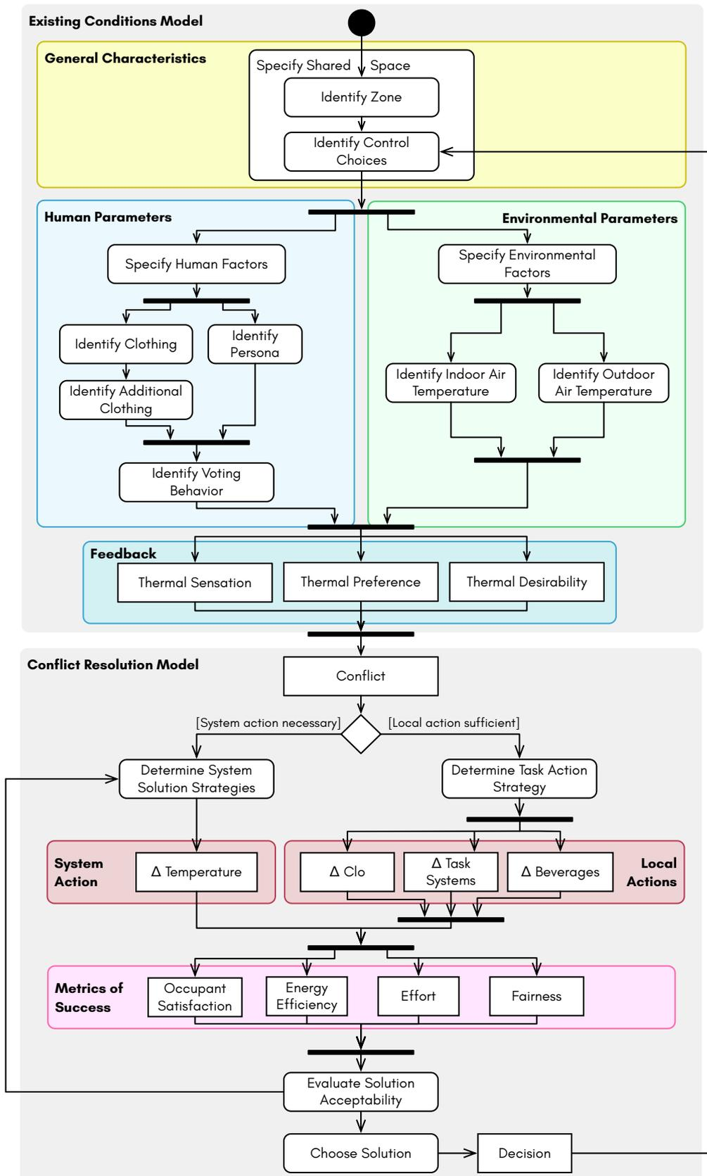
Figure 6.1: Simulation Process Model (UML Activity Diagram)
