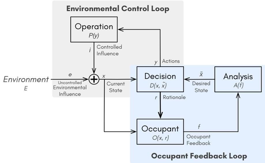
Figure 3.3: **Causal Non-linear MIMO Control System** with two feedback loops (Block Diagram)
