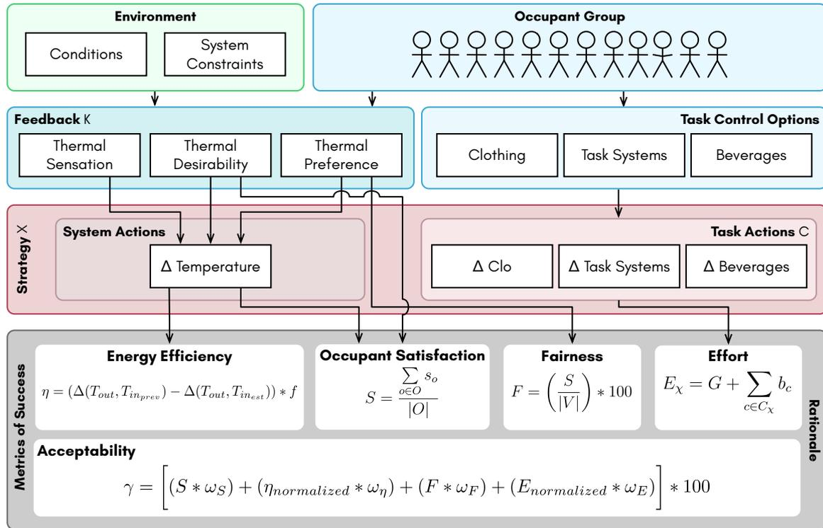
Figure 6.3: Input Parameters, Actions, and Metrics of Success for Negotiated Thermal Control
