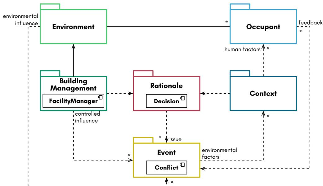
Figure 3.4: **High-level View of TREATI** organized into six packages (UML Package Diagram)
