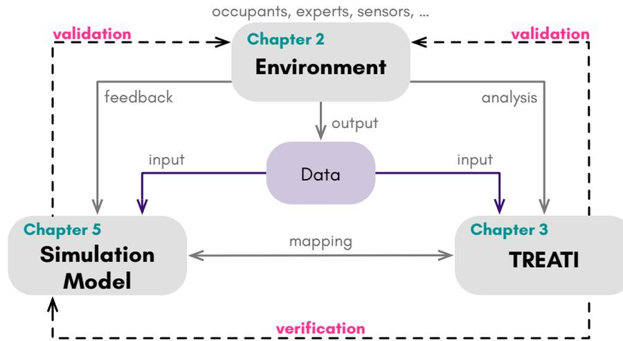
Figure 1.2: **Validation Model** – The **Simulation Model** uses the real-world environmental data to test scenarios and identify errors. These are then rectified in **TREATI** and are reconciled with the simulation model. The validation model is based on the work from Robert G. Sargent [Sar99] and Donald A. Norman and Stephen W. Draper [ND86]
