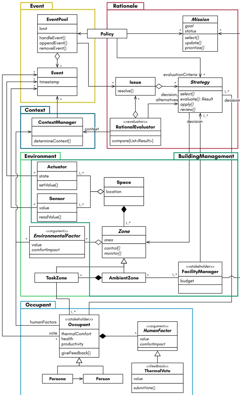
Figure 3.12: The detailed **TREATI Object Model** consists of six packages and the associations between them (UML Class Diagram)
