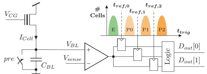
Fig. 1. Simplified schematic of the time-domain voltage sensing applied on a distribution of four cell states (E, P0, P1, P2)
