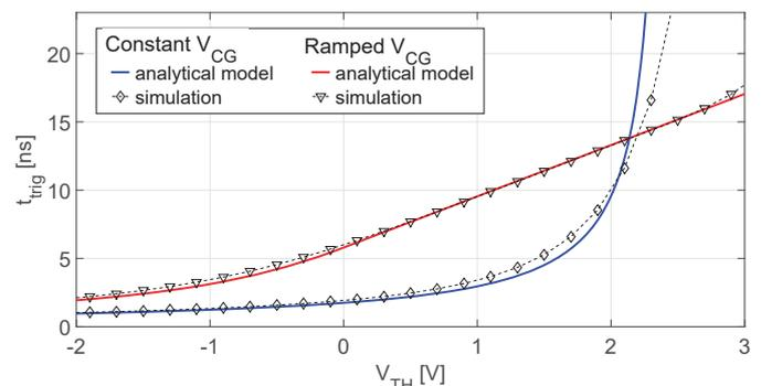
Fig. 2. Transfer characteristic from cell threshold to trigger time obtained by an analytical model and by simulation. Diamonds: constant  $V_{CG} = 2.5V$ , Triangles: linear voltage ramp starting from 0 V with slope  $s = 260 \text{ mV/ns}$
