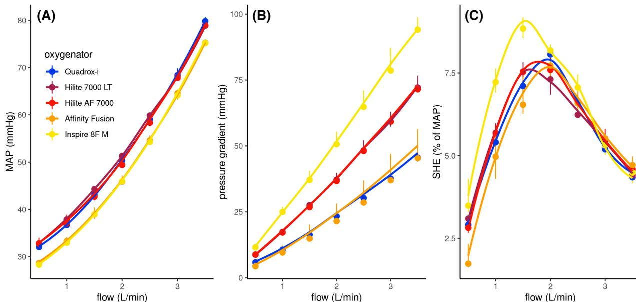
**FIGURE 3** Flow dependence of mean arterial pressure (MAP, panel A), the pressure gradient across the oxygenator (B), and surplus hemodynamic energy (SHE, panel C) normalized to MAP during pulsatile flow (frequency  $50 \text{ min}^{-1}$ , systolic duration 50%, rotational speed gain  $2300 \text{ min}^{-1}$ ) with a single DP3 diagonal pump. Colors indicate the type of oxygenator.  $n = 6$ .
