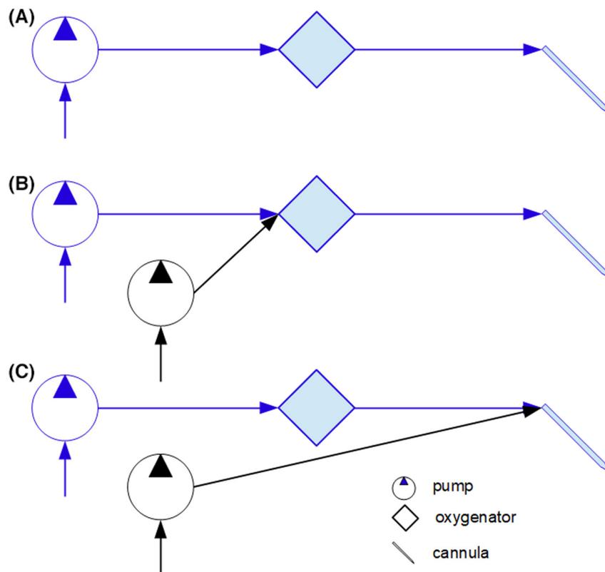
**FIGURE 2** Schematic diagrams of alternative extracorporeal circulation setups. (A) Default setup using a single DP3 pump (cf. Figure 1), (B and C) setups using two parallel synchronized DP3 pumps, (B) both pumps fed the oxygenator, and (C) one pump bypassed the oxygenator.
