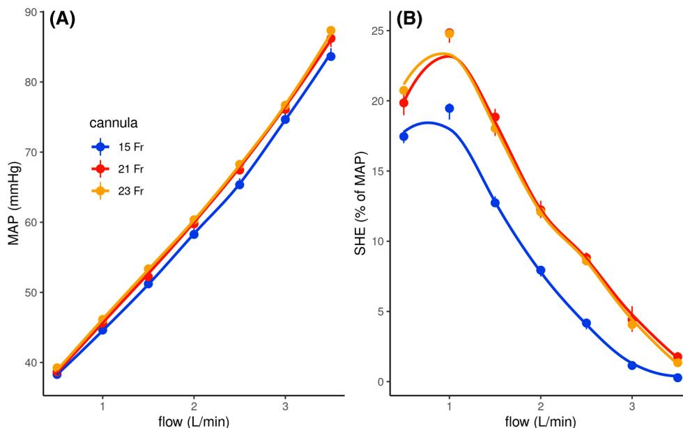
**FIGURE 5** Flow dependence of mean arterial pressure (MAP, panel A) and surplus hemodynamic energy (SHE, panel B) normalized to MAP during pulsatile flow (frequency  $40 \text{ min}^{-1}$ , systolic duration 35%, rotational speed gain  $2500 \text{ min}^{-1}$ ) with a single DP3 diagonal pump. Colors indicate the gauge of the cannula.  $n = 6$ .
