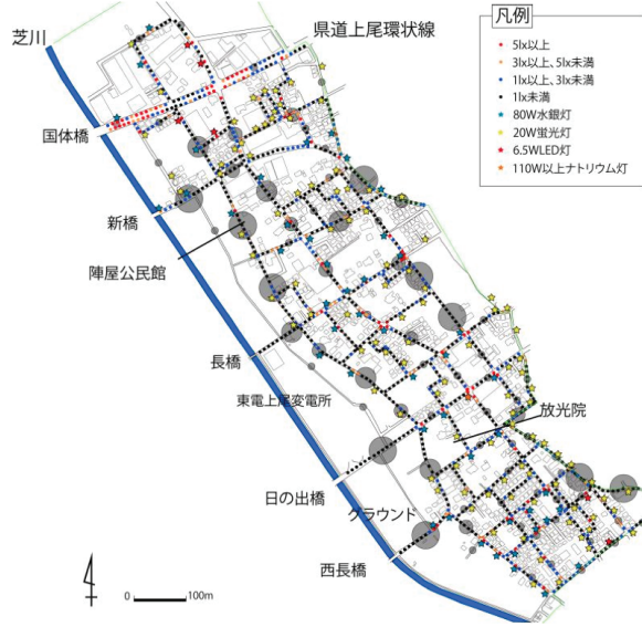
Figure 2.2. An example of mapping brightness of road at night [16].
