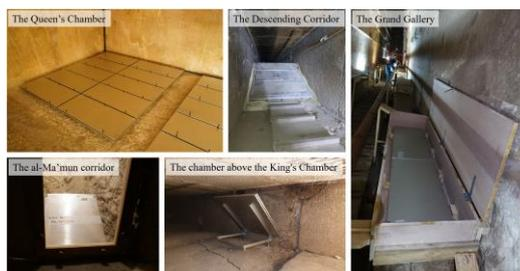
*Figure 2: Nuclear emulsion detectors installed in the Pyramid of Khufu.*
