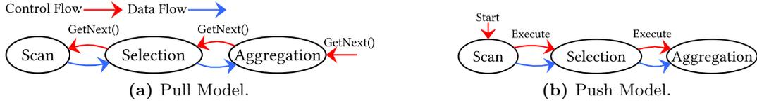
**Figure 2.3:** Illustration of the **pull-(a)** and **push-(b)** query execution model for a scan, select, aggregate query.
