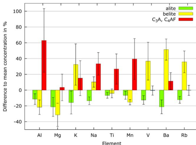
**Figure 2** Difference to the mean element concentration for each phase. Concentration data originate from three experiments on the same sample. Segmentation was done using the respective EDX datasets. Only the segmented areas of alite, belite and  $\text{C}_3\text{A}/\text{C}_4\text{AF}$  were considered for the mean value. The error bars represent the standard deviation of an element concentration within a phase.
