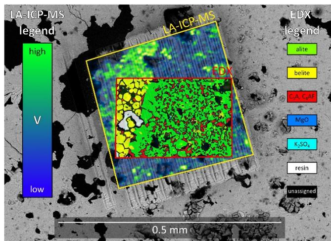
**Figure 1** Illustration of the main concept. A SEM-BSE image is combined with a SED-EDX-phase mapping and the respective LA-ICP-MS dataset to allocate minor and trace elements to identified phases.
