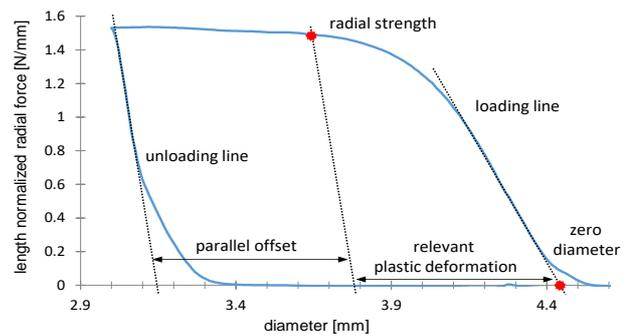
**Figure 2:** Representative radial force curve of a balloon expandable stent using a segmented head test setup
