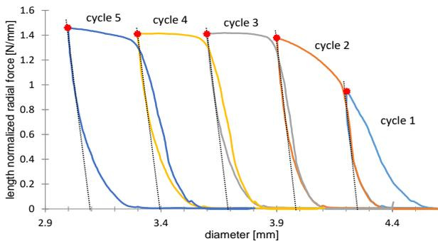
**Figure 3:** Representative radial force curves for a multi-cycle measurement with different slopes of the unloading lines (dotted lines) as well as peak forces (red dots)
