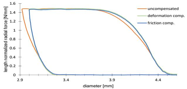
**Figure 4:** Comparative illustration of radial force curve progression of a balloon expandable stent with and without compensation of deformation as well as friction within the test segmented head test mechanism
