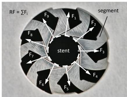
**Figure 1:** Test principle of radial force testing of a vascular stent via segmented head test mechanism, total radial force represents the sum of reaction forces at each segment
