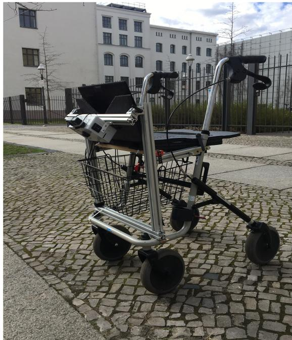
**Figure 4.6:** Prototype with the customized foundation and sensors
