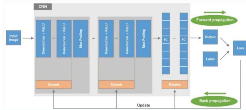
Figure 2.14: An overview of the training procedure and a convolutional neural network (CNN) architecture (Adapted from [62]).
