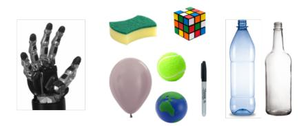
Figure 5.26.: Soft-grasping problem definition. Given a limited number of hand primitives, adapt them to grasp objects with different shapes, stiffness and sizes without knowing their exact geometric and physical properties. Use compliant control without force sensors to control a real anthropomorphic robot hand.
