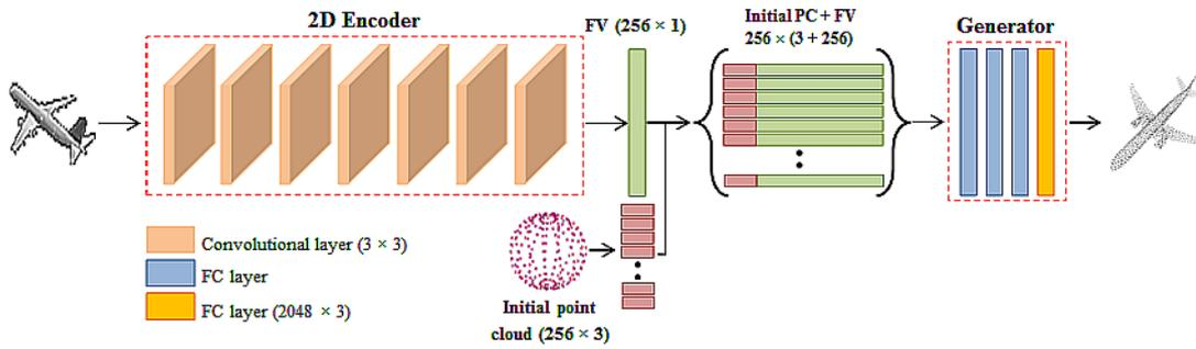
**Figure 5.3:** The proposed CNN Architecture. The encoder network extracts features from the input image. The extracted feature vector is concatenated with the coordinates of the sphere points. The generator takes the extracted feature vector and the coordinates of the sphere as input and generates the final point cloud of the input object.
