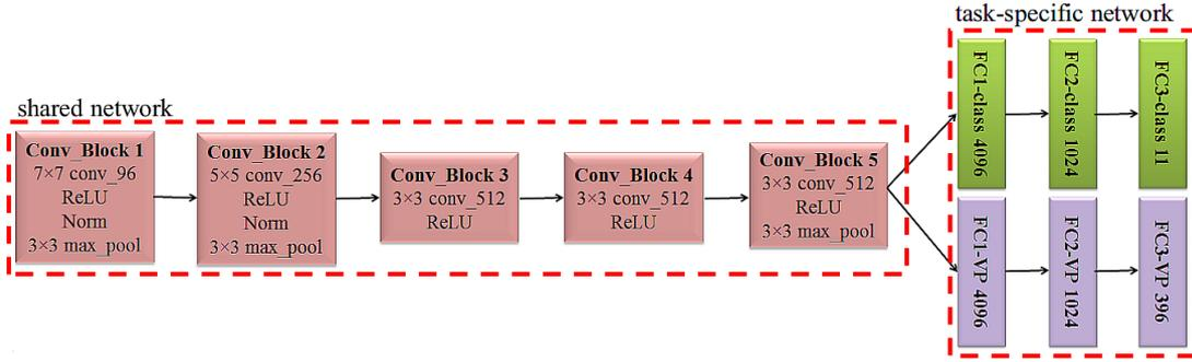
**Figure 3.3:** The proposed CNN architecture. ReLU is the activation function we use for the nonlinearity. Max-pooling is used in the first, second, and fifth convolutional blocks. The FC viewpoint output layer is an object category dependent layer. FC layers are followed by a dropout layer with a rate of 0.5.
