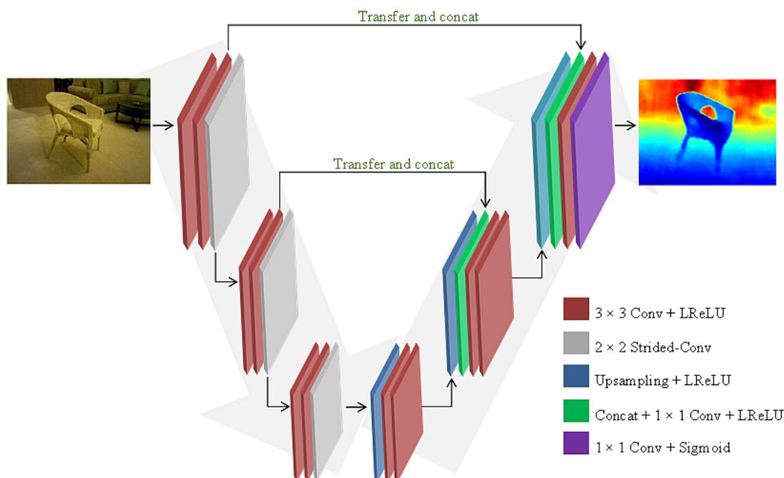
**Figure 4.2:** mini strided V-Net architecture. Pooling layers are replaced by strided-convolutional layers to generate an output of the same resolution as that of the input.
