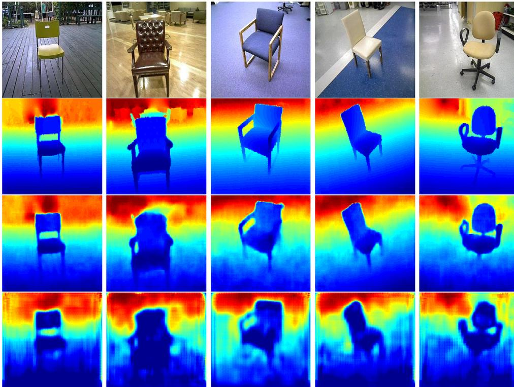
**Figure 4.8:** Qualitative comparison results on Large Dataset of Object Scans using different loss functions on mini V-Net model. From top to bottom: input RGB image, ground-truth, model trained using Tukey’s biweight loss, model trained using L2 norm. Depths are shown in log scale and in color (blue is close, red is far).
