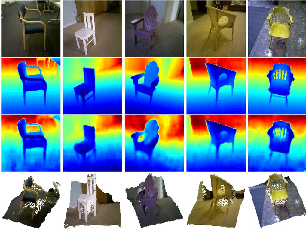
**Figure 4.6:** Qualitative results from mini V-Net on Large Dataset of Object Scans (chosen from the testing set). From top to bottom: input RGB image, ground-truth, predicted depth image, and the reconstructed images using the predicted depth values. Depths are shown in log scale and in color (blue is close, red is far).
