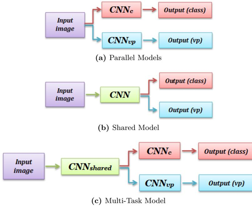
**Figure 3.2:** Different network setups for joint object classification and viewpoint estimation. (a) Independent and parallel models for each task. (b) A shared model for both tasks and the output layer splits into two layers; one for each task. (c) A multi-task model that has a shared network and branches into two networks; one for each task.
