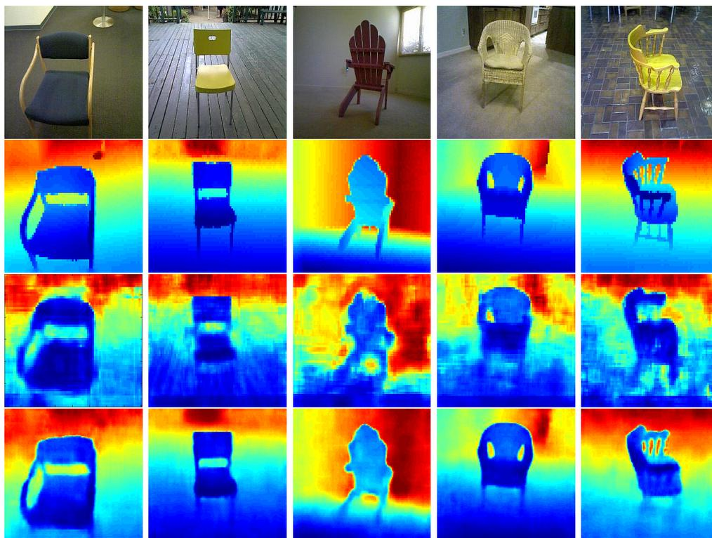
**Figure 4.9:** Qualitative comparison results on Large Dataset of Object Scans. From top to bottom: input image, ground-truth, F-CNN trained on Tukey’s biweight loss, and mini V-Net trained on Tukey’s biweight loss. Depths are shown in log scale and in color (blue is close, red is far).
