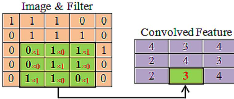
Figure 2.2: A convolutional operation with a  $3 \times 3$  filter.
