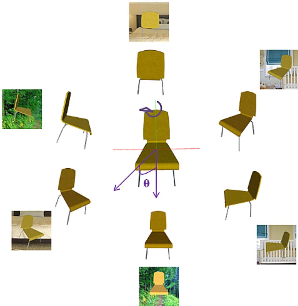
**Figure 3.4:** Preparing the training data. We render many images from the synthetic 3D models from different orientations. The rendered images are overlaid with real background to mimic the real data.
