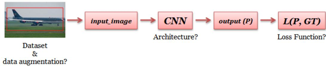
**Figure 1.1:** An overview of the challenges appeared when proposing a deep learning model.  $L$  is the loss function,  $P$  is the predicted output, and  $GT$  is the ground-truth.
