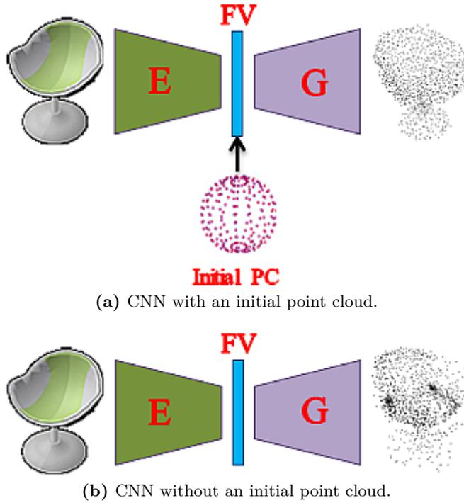
**Figure 5.6:** A general sketch of the proposed CNN model with different setups. (a) the proposed CNN with an initial point cloud. (b) the proposed CNN without the initial point cloud. E: Encoder, G: Generator, PC: Point Cloud, FV: Feature Vector.
