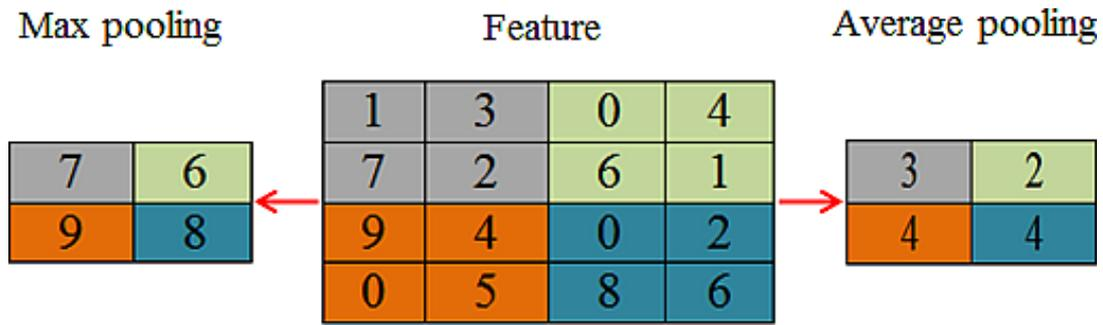
**Figure 2.4:** Different Pooling Operations with  $2 \times 2$  filters and stride 2.
