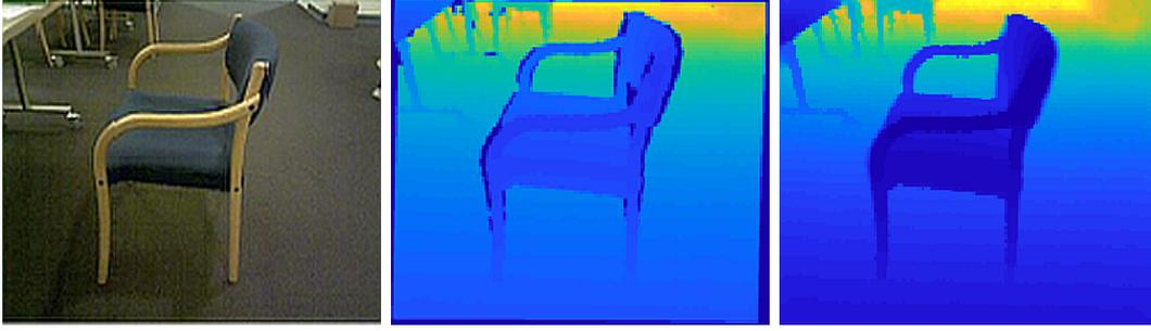
**Figure 4.4:** A sample of a training RGB image with the corresponding depth image. From left to right: RGB image, original depth image, and preprocessed depth image.
