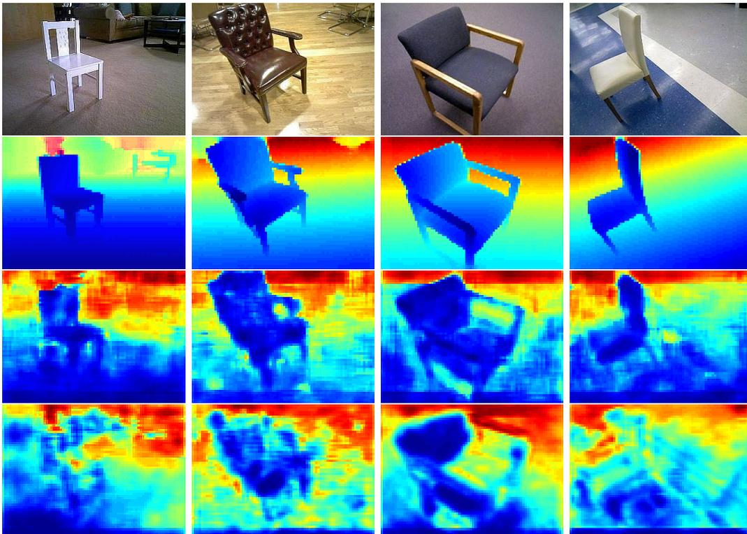
**Figure 4.5:** Qualitative results from F-CNN on Large Dataset of Object Scans (chosen from the testing set). From top to bottom: input RGB image, ground-truth, results from the model trained on Tukey’s biweight loss, and results from the model trained on L2 norm. Depths are shown in log scale and in color (blue is close, red is far).
