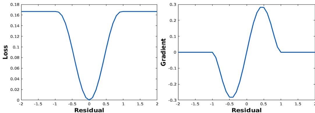
**Figure 4.3:** Tukey’s biweight loss function (left) and its first-order derivative (right) where  $c = 1$ .
