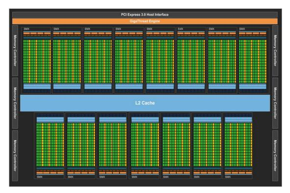
Figure 4.7: NVIDIA K40c GPU GK110 Architecture
