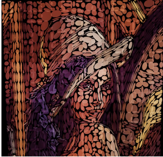
Figure 1.6: Illustration of the kernels in a SMoE model of the standard test image Lena. Each kernel describes a region in the 2-D coordinate space and a gradient in the 3-D color space. Note that kernels have theoretical global support, however, the kernels are cut off for illustration purposes.
