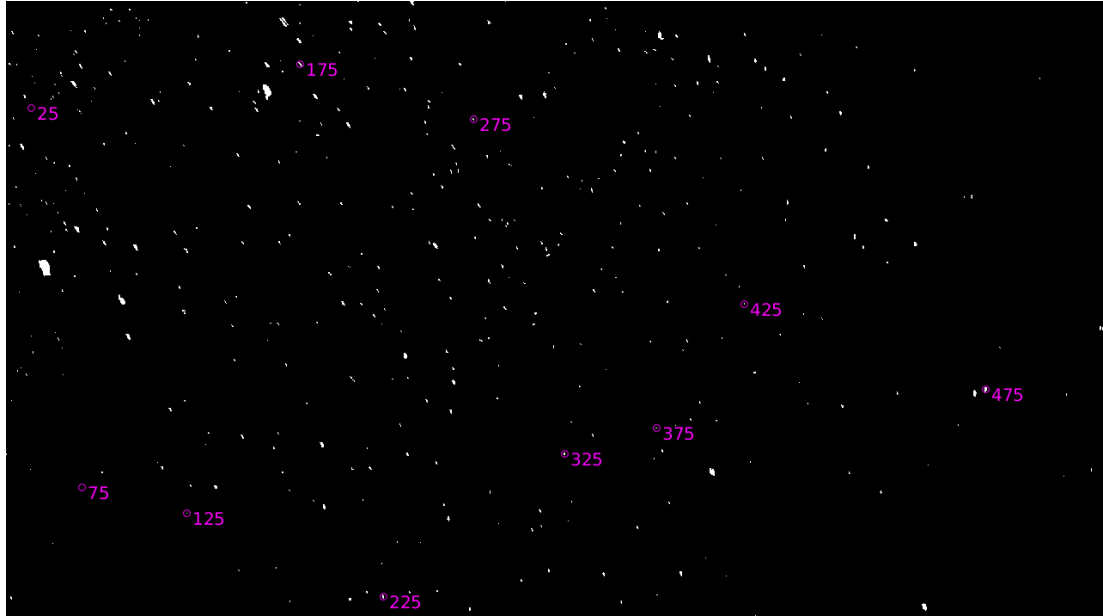
Figure 3.6: Tracer particles represented with pixels in 1 – bit monochrome space
