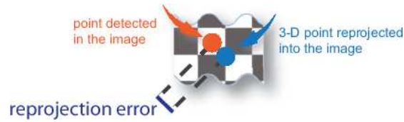
Figure 5.2: Graphical Representation of Reprojection Error [31]
