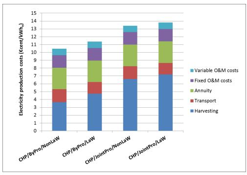
Figure 8.1: Cost breakdown of the electricity production costs incurred by the CHP-based power plant (20 MW<sub>e</sub>) for the four resources-related compound scenarios
