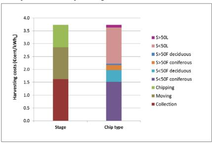
Figure 7.37: Cost component split of harvesting costs on the basis of both the harvesting stages and the types of wood chips for the supply chain of a BIGCC-based power plant of 340 MW<sub>e</sub>
