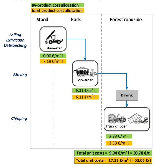
Figure 3.5: Techno-economic breakdown of the fully mechanised logistic chain of chipped forest residues for an average DBH of 15 cm and 35% MC according to both cost allocation procedures either as a by-product or as a joint product
