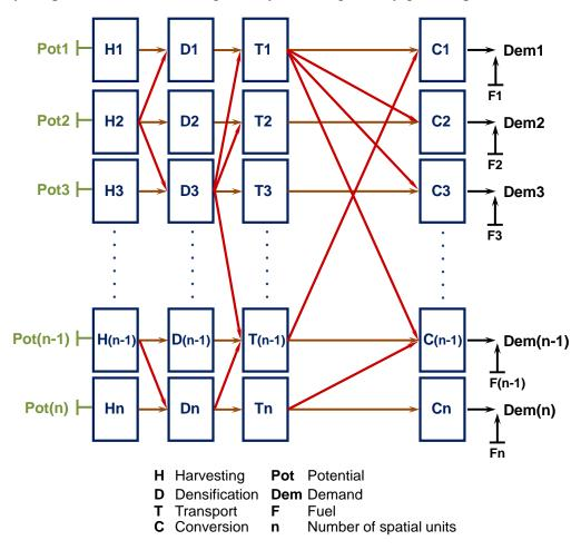
Figure 5.2: Structure of the BIOSPHERE model as a grid of producers connected by energy flows for a bioenergy system composed of n spatial units
