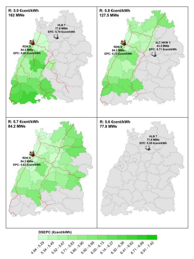
Figure 7.40: Location and EPC of retrofitted coal power plants in addition to catchment area illustrating the corresponding DSEPC for the RDK 8 facility as a function of the remuneration R (5.6, 5.7, 5.8 and 5.9  $\in$  cent/kWh<sub>e</sub>)
