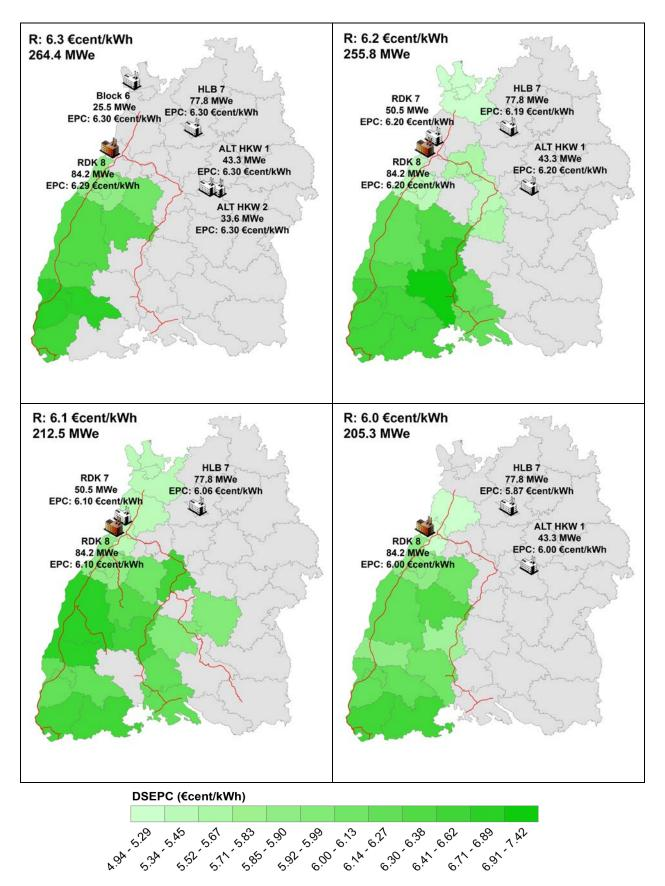
Figure 7.39: Location and EPC of retrofitted coal power plants in addition to catchment area illustrating the corresponding DSEPC for the RDK 8 facility as a function of the remuneration R (6, 6.1, 6.2 and 6.3  $\in$  cent/kWh<sub>e</sub>)
