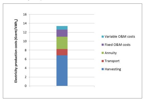
Figure 7.11: Cost breakdown of the electricity production costs of a representative FBG+E-based power plant of 20  $MW_e$  into their cost elements
