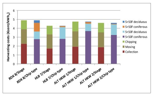
Figure 7.21: Cost component split of harvesting costs on the basis of both the harvesting stages and the types of wood chips for the supply chains of the co-firing based RDK 8, HLB 7, ALT HKW 1 and ALT HKW 2 power plants
