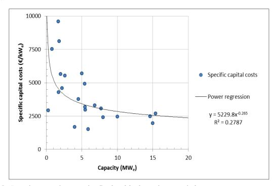
Figure 4.5: Specific capital costs of a fluidised bed gasifier coupled to a gas engine as a function of the electric capacity
