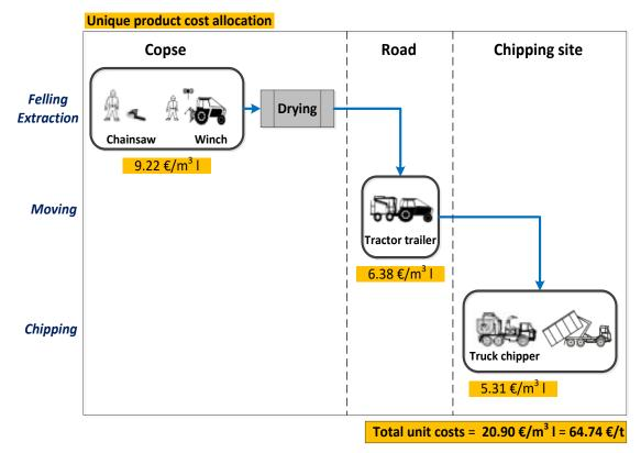
Figure 3.6: Techno-economic breakdown of the partly mechanised logistic chain of chipped landscape wood raw material as a unique product for an average DBH of 10 cm and 35% MC
