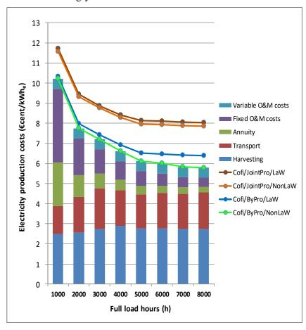
Figure 7.25: Dependence of specific electricity production costs and their cost components on the full load hours for the RDK 8 conversion unit in each of the four cofiring compound scenarios
