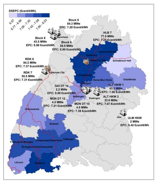
Figure 7.16: Location of the selected co-firing based coal power plants as well as illustration of the catchment areas of RDK 8 and HLB 7 respectively with their corresponding EPC and DSEPC in each specific district
