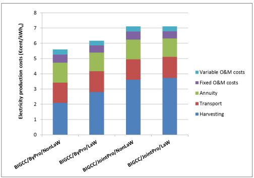
Figure 8.3: Cost breakdown of the electricity production costs incurred by the BIGCC-based power plants (210/340 MW<sub>e</sub>) for the four resources-related compound scenarios
