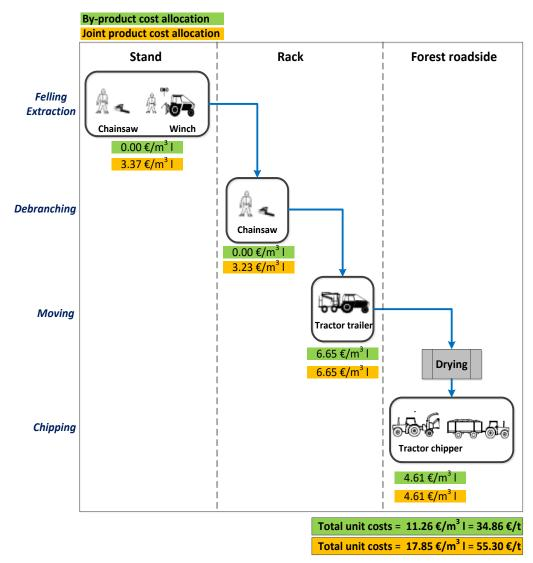
Figure 3.2: Techno-economic breakdown of the motor-manual logistic chain of chipped forest residues for an average DBH of 15 cm and 35% MC on the basis of both cost allocation procedures either as a by-product or as a joint product<sup>16</sup>
