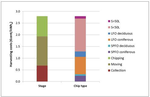
Figure 7.31: Cost component split of harvesting costs on the basis of both the harvesting stages and the types of wood chips for the supply chain of a BIGCC-based power plant of 340 MW<sub>e</sub>
