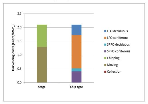
Figure 7.28: Cost component split of harvesting costs on the basis of both the harvesting stages and the types of wood chips for the supply chain of a BIGCC-based power plant of 210 MW<sub>e</sub>
