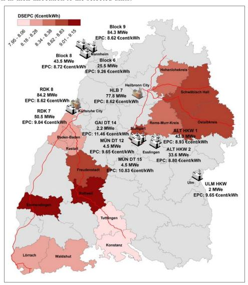
Figure 7.22: Location of the selected co-firing based coal power plants as well as illustration of the catchment areas of RDK 8 and HLB 7 respectively with their corresponding EPC and DSEPC in each specific district
