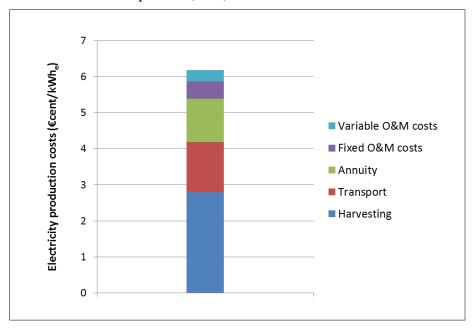
Figure 7.30: Cost breakdown of the electricity production costs incurred by the BIGCC-based power plant of 340 MW<sub>e</sub> into their cost elements
