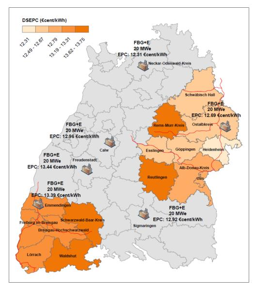
Figure 7.7: Location of the six FBG+E-based power plants with the respective EPC along with two representative catchment areas illustrating the DSEPC in the corresponding administrative units
