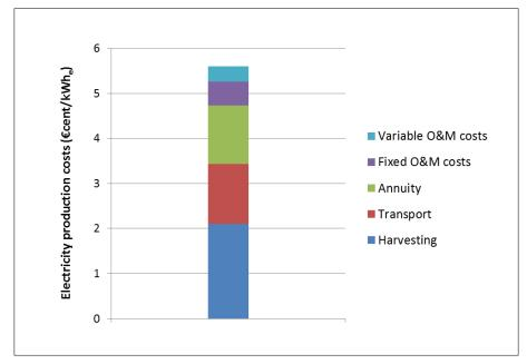
Figure 7.27: Cost breakdown of the electricity production costs incurred by the BIGCC-based power plant of 210 MW<sub>e</sub> into their cost elements
