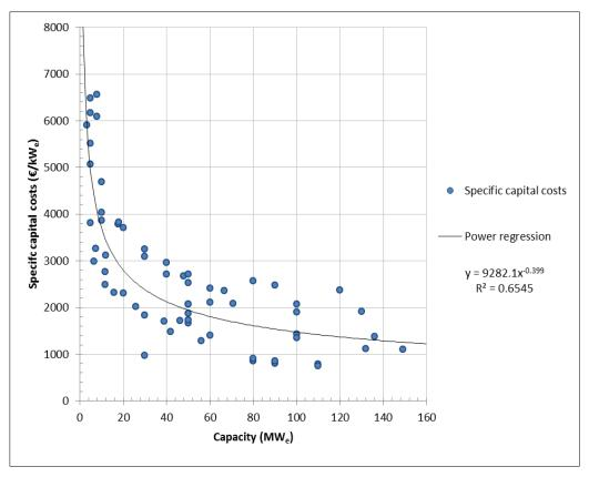
Figure 4.9: Specific capital costs of a fluidised bed gasifier coupled to a combined cycle as a function of the electric capacity
