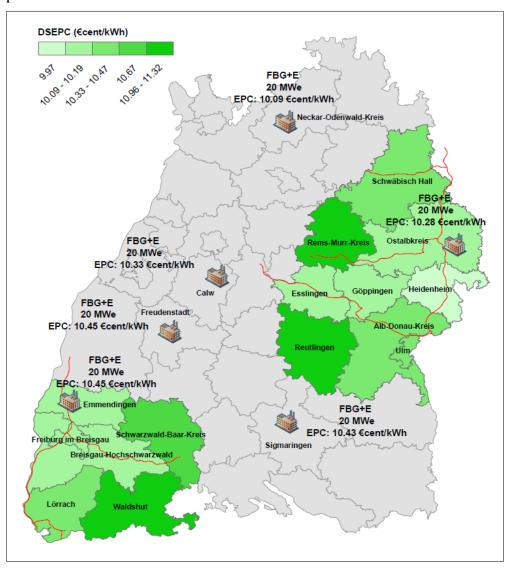
Figure 7.1: Location of the six FBG+E-based power plants with the respective electricity production costs along with two representative catchment areas illustrating the district-specific electricity production costs in the corresponding administrative units
