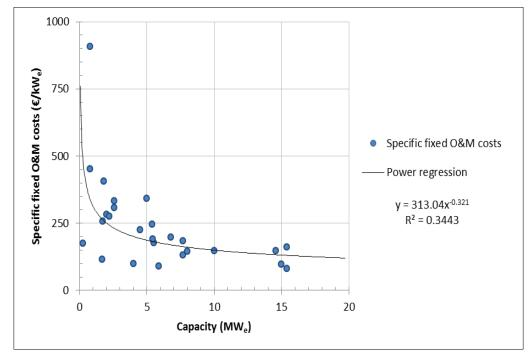
Figure 4.6: Specific fixed O&M costs of a fluidised bed gasifier coupled to a gas engine as a function of the electric capacity
