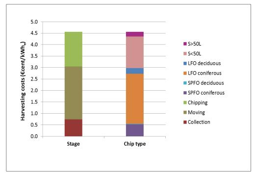
Figure 7.6: Cost component split of harvesting costs on the basis of both the harvesting stages and the types of wood chips for the supply chain of a representative FBG+E-based power plant of 20 MW<sub>e</sub>
