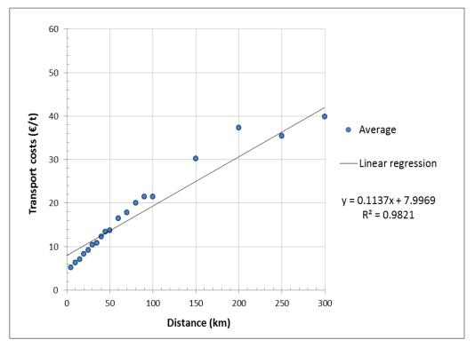
Figure 3.9: Linear regression of averaged transport costs versus the covered distance
