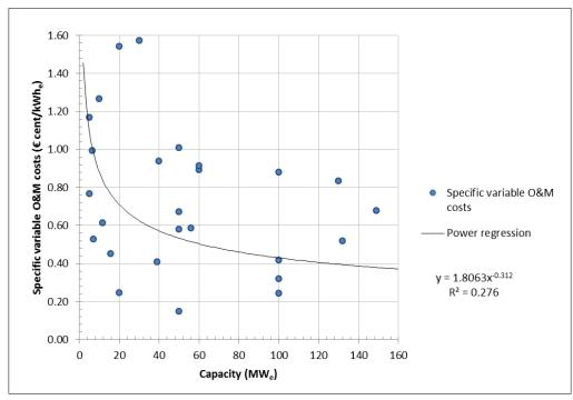
Figure 4.11: Specific variable O&M costs of a fluidised bed gasifier coupled to a combined cycle as a function of the electric capacity
