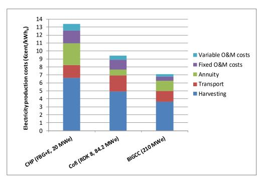
Figure 8.6: Cost breakdown of the electricity production costs incurred by the bio-based power plants of the three technology settings within the resources-related compound scenario of forest residues as a joint product
