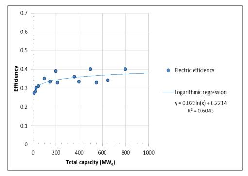
Figure 4.4: Electric efficiency of co-firing for a 10% fraction of wood resources as a function of the total electric capacity
