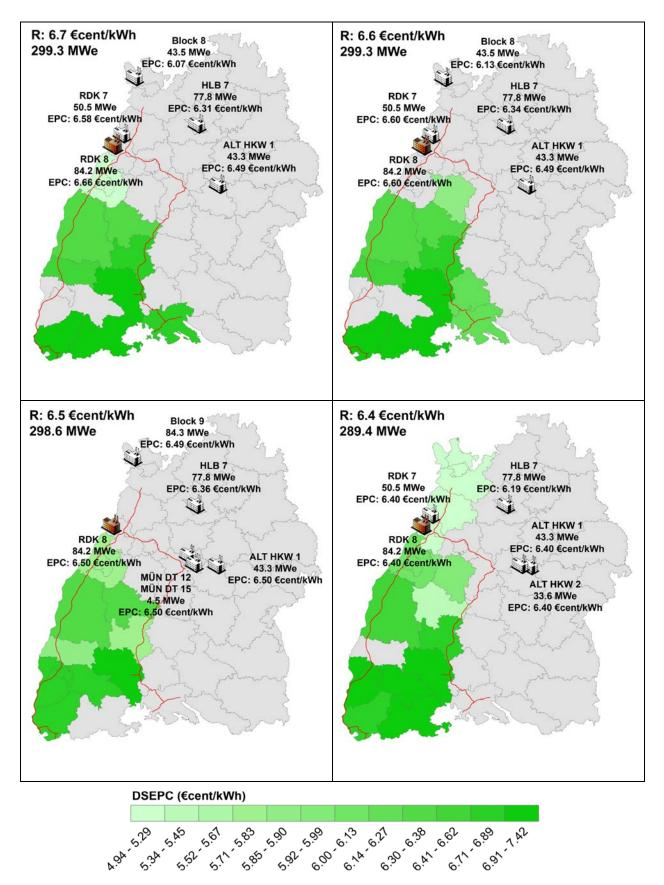
Figure 7.38: Location and EPC of retrofitted coal power plants in addition to catchment area illustrating the corresponding DSEPC for the RDK 8 facility as a function of the remuneration R (6.4, 6.5, 6.6 and 6.7  $\in$  cent/kWh<sub>e</sub>)
