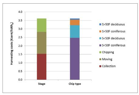
Figure 7.34: Cost component split of harvesting costs on the basis of both the harvesting stages and the types of wood chips for the supply chain of a BIGCC-based power plant of 210 MW<sub>e</sub>
