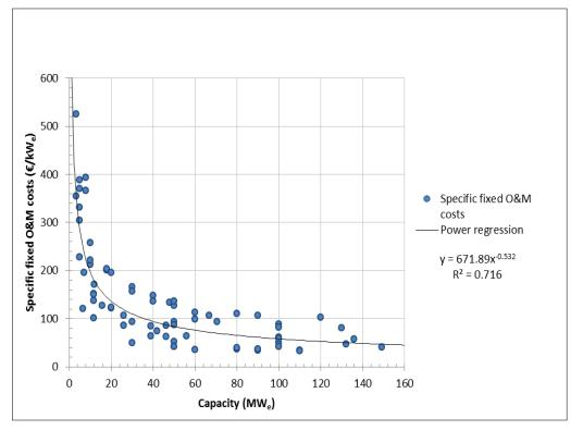
Figure 4.10: Specific fixed O&M costs of a fluidised bed gasifier coupled to a combined cycle as a function of the electric capacity
