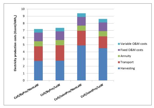
Figure 8.2: Cost breakdown of the electricity production costs incurred by the co-firing based power plant (RDK 8, 84.2 MW<sub>e</sub>) for the four resources-related compound scenarios
