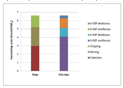
Figure 7.9: Cost component split of harvesting costs on the basis of both the harvesting stages and the types of wood chips for the supply chain of a representative FBG+E-based power plant of 20 MW<sub>e</sub>
