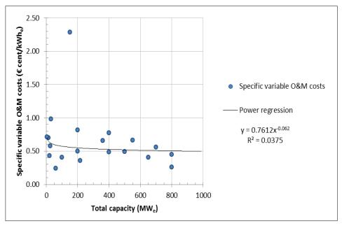
Figure 4.3: Specific variable O&M costs of co-firing for a 10% fraction of wood resources as a function of the total electric capacity
