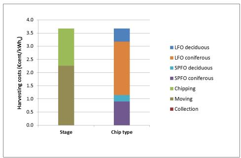
Figure 7.3: Cost component split of harvesting costs on the basis of both the harvesting stages and the types of wood chips for the supply chain of a representative FBG+E-based power plant of 20 MW<sub>e</sub>
