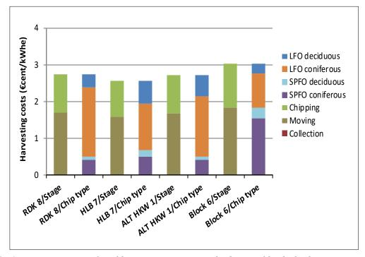
Figure 7.15: Cost component split of harvesting costs on the basis of both the harvesting stages and the types of chipped forest residues for the supply chains of the co-firing based RDK 8, HLB 7, ALT HKW 1 and Block 6 power plants
