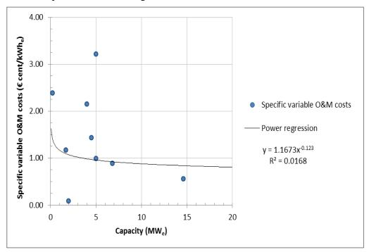
Figure 4.7: Specific variable O&M costs of a fluidised bed gasifier coupled to a gas engine as a function of the electric capacity
