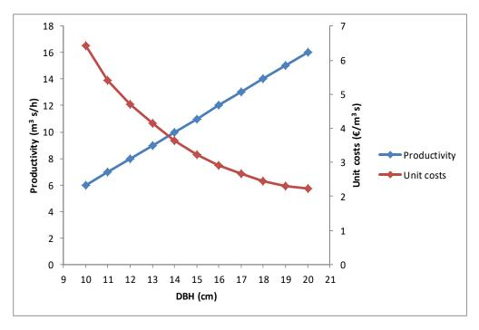
Figure 3.1: Correlation between productivity and unit costs for the motor-manual felling of trees versus their increasing diameter at breast height (based on [Hepperle 2010]) ( $m^3$  s ~ cubic meter solid volume)
