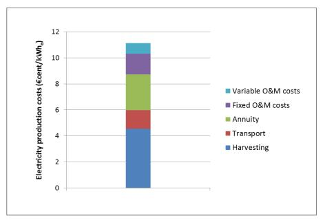
Figure 7.5: Cost breakdown of the electricity production costs of a representative FBG+E-based power plant of 20 MW<sub>e</sub> into their cost elements
