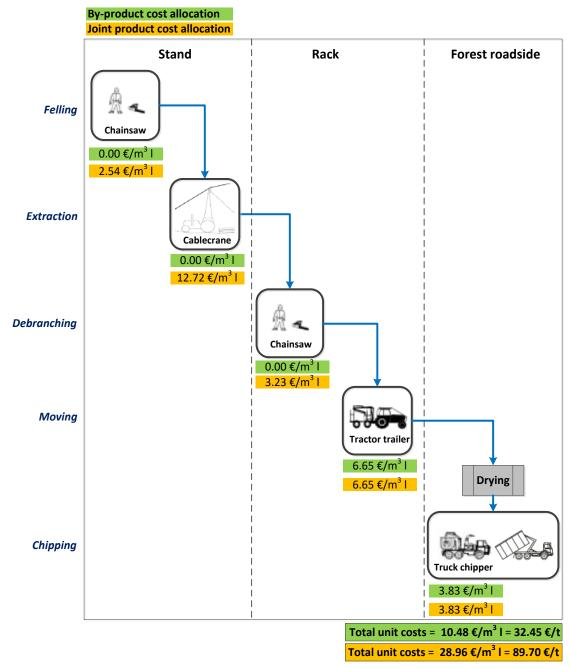
Figure 3.4: Techno-economic breakdown of the highly mechanised logistic chain of chipped forest residues for an average DBH of 15 cm and 35% MC on the basis of both cost allocation procedures either as a by-product or as a joint product
