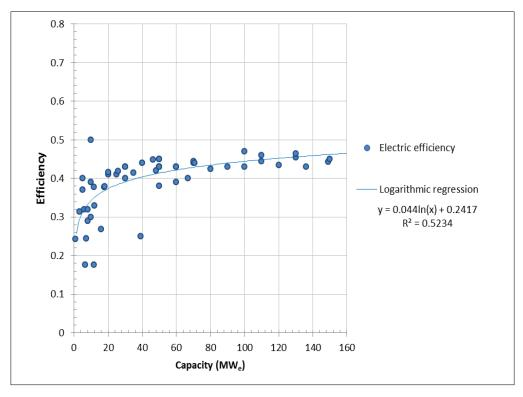
Figure 4.12: Electric efficiency of a fluidised bed gasifier coupled to a combined cycle as a function of the electric capacity
