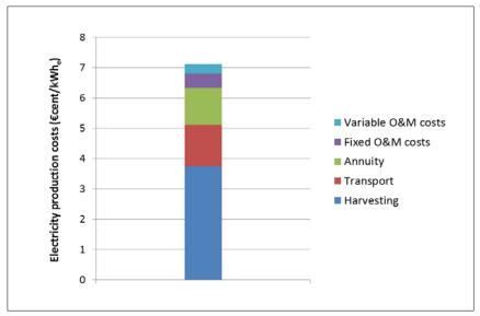
Figure 7.36: Cost breakdown of the electricity production costs incurred by the BIGCC-based power plant of 340 MW<sub>e</sub> into their cost elements
