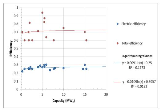
Figure 4.8: Electric and total efficiency of a fluidised bed gasifier coupled to a gas engine as a function of the electric capacity
