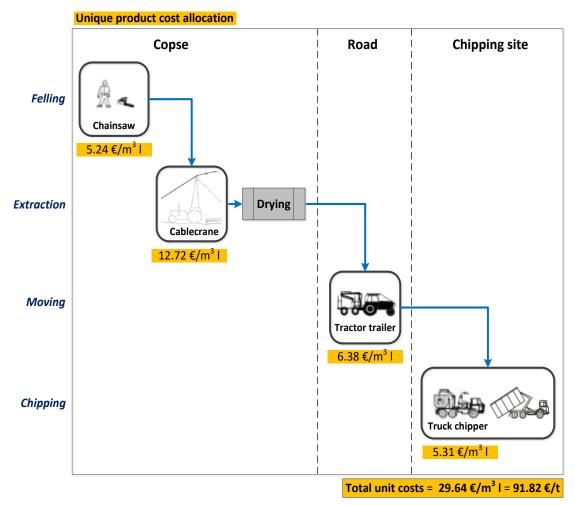
Figure 3.7: Techno-economic breakdown of the highly mechanised logistic chain of chipped landscape wood raw material as a unique product for an average DBH of 10 cm and 35% MC
