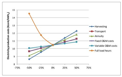
Figure 7.41: Two-dimensional sensitivity analysis of specific electricity production costs when varying the respective cost components and the full load hours for the CHP/ByPro/NonLaW compound scenario
