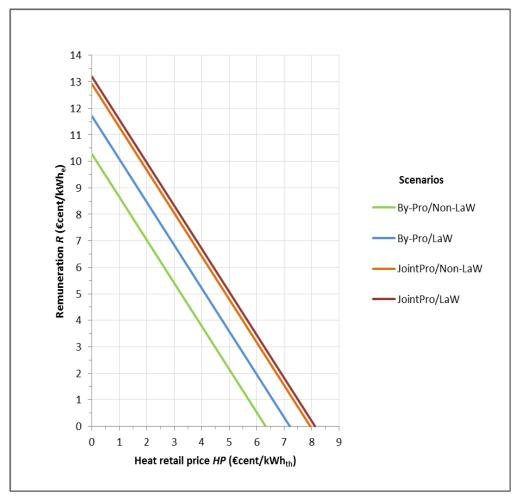
Figure 8.9: Remunerations and heat retail prices granted to a CHP facility based on a fluidised bed gasifier connected to a gas engine of 20 MW<sub>e</sub> as monetary amounts minimally required for the investment to break even within the four wood resources-related compound scenarios
