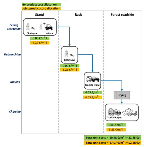
Figure 3.3: Techno-economic breakdown of the partly mechanised logistic chain of chipped forest residues for an average DBH of 15 cm and 35% MC according to both cost allocation procedures either as a by-product or as a joint product
