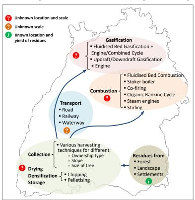
Figure 1.1: Value chain of wood resources for power generation in Baden-Württemberg including all the utilisation pathways as a combination of consecutive processes with different location, technology and scale
