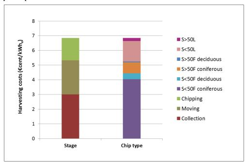
Figure 7.12: Cost component split of harvesting costs on the basis of both the harvesting stages and the types of wood chips for the supply chain of a representative FBG+E-based power plant of 20 MW<sub>e</sub>
