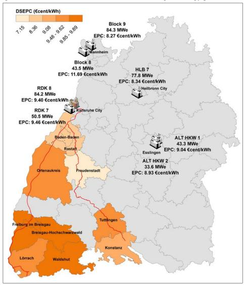
Figure 7.19: Location of the selected co-firing based coal power plants as well as illustration of the catchment area of RDK 8 respectively with their corresponding EPC and DSEPC in each specific district
