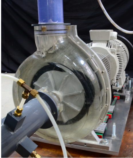
Figure 6.2: The vortex pump used for the tests (left) and its cross section view (right; both taken from Gerlach et al. [48]).
