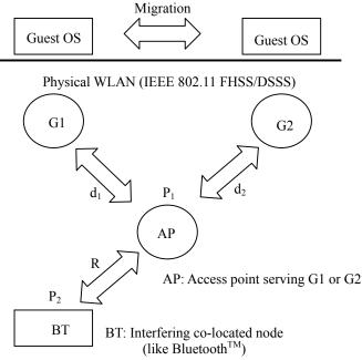
**Figure 2:** An interference scenario of OS migration set on a WLAN-link. The RF interference (RFI) is presumably caused by an IEEE 802.11 FHSS/DSSS device (like Bluetooth<sup>TM</sup>) communication. R, d<sub>1</sub>, and d<sub>2</sub> are node separations (in meter) as shown, P<sub>1</sub> and P<sub>2</sub> are transmitted power levels of the units.
