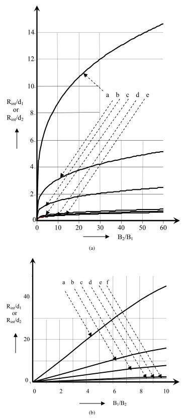
**Figure 4:**  $B_1/B_2$  ratio (>1) *versus*  $R_{int}$  (normalized with respect to  $d_1$  or  $d_2$ ) for a set of parametric values of the probability of bit-error (BER). The graphs shown correspond to  $P_e = \{0.0001, 0.0010, 0.0050, 0.0500, 0.0750, 0.1000\} \equiv \{a, b, c, d, e, f\}$ ; (a)  $B_1/B_2$  ratio over a range of 0 to 600, (b)  $B_1/B_2$  ratio over a range of 0 to 10.
