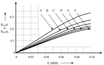
**Figure 3:**  $R_{int}$  (normalized with respect to  $d_1$  or  $d_2$ ) *versus* the probability of biterror (BER) for a set of parametric values,  $B_1/B_2$ . The graphs shown correspond to the following sets:  $B_1/B_2 = \{1/100, 1/200, 1/300, 1/400, 1/500, 1/600\} \equiv \{A, B, C, D, E, F\}$ .
