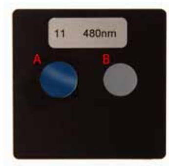
**Figure 3.1:** One of 39 camSPECS filter plates.
