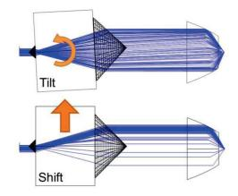
Fig. 3 Introduction of coma aberration (top) and non-symmetric intensity profile (bottom).
