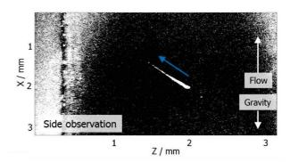
Fig. 4 Side view on trapped particle and particle movement (blue arrow) due to shift of DA.
