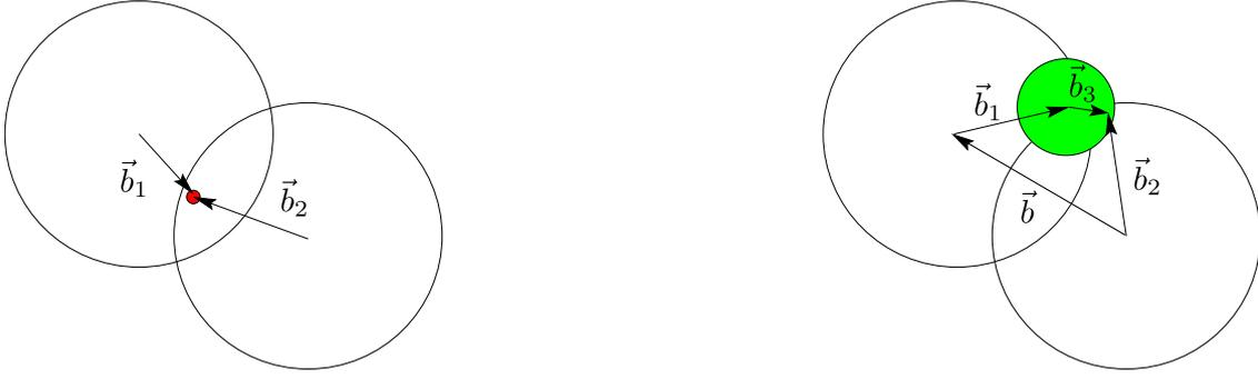
Figure 3.2: Profile overlap in case of hard (left) and soft (right) interactions.
