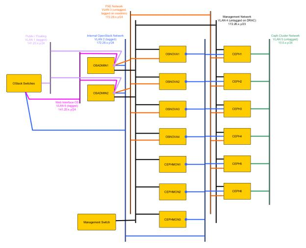
Figure 2. OpenStack physical testbed topology at HU
