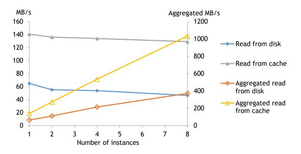
Figure 3. Read performance for sequential reads depending on number of instances.
