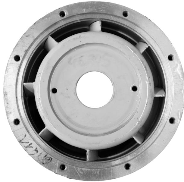
**Figure 4.17:** Oil pump housing partial view with flow guiding blades [113].
