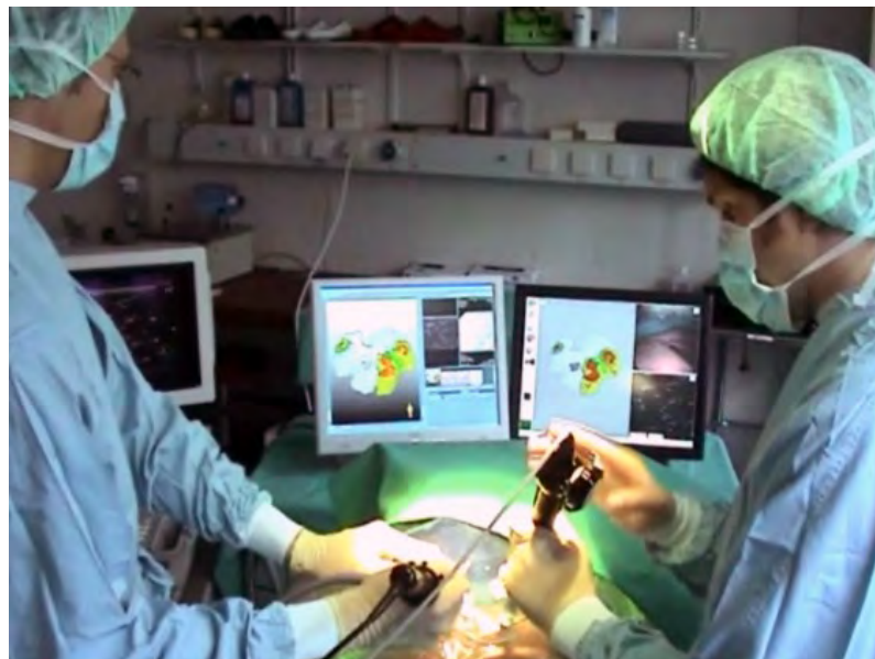
Figure 4.9: Evaluation of the IPA within an experimental operating room (Institute of Biomedical Optics, University of Lübeck, Germany) using a tumor mimic model. The left screen belongs to the IPA; the right screen belongs to the navigation system.
