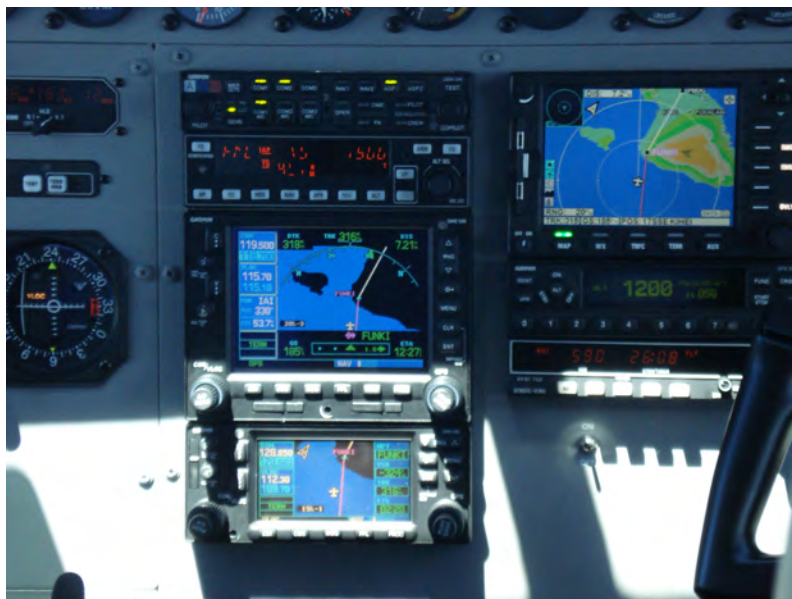
Figure 5.1: Maps in the cockpit of an aircraft during the approach of a mountainous island. The topographic map in the upper right visualizes the position of the aircraft and the location and height of surrounding mountains.
