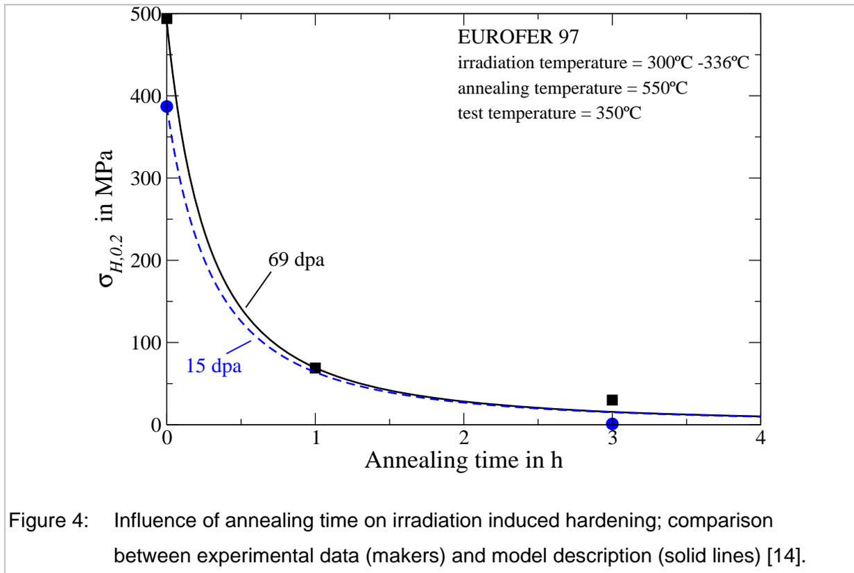
Figure 4: Influence of annealing time on irradiation induced hardening; comparison between experimental data (makers) and model description (solid lines) [14].
