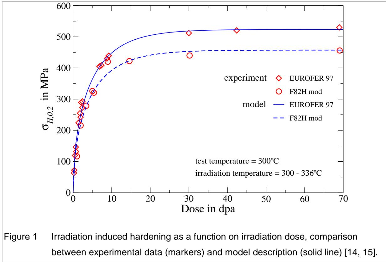
Figure 1 Irradiation induced hardening as a function on irradiation dose, comparison between experimental data (markers) and model description (solid line) [14, 15].
