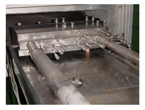
Figure 11: Module installed in the liquid metal loop. The pressure taps are still closed by caps in this stage of installation.
