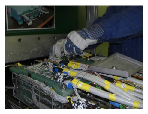
Figure 23: Reconnection of some pressure lines which had been disconnected for installation of insulating plates carrying potential sensors.
