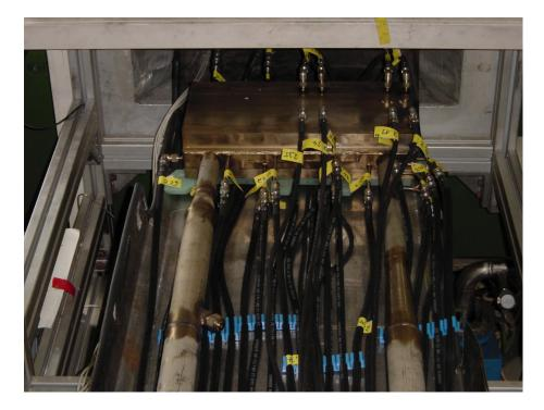
Figure 19: Connection of pressure taps with pressure transducers through flexible rubber tubes.
