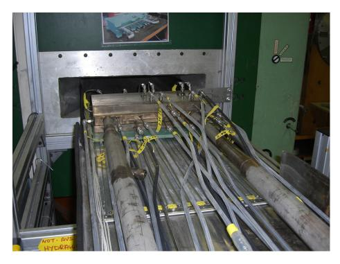
Figure 20: Connection of pressure taps with pressure transducers through rigid pipes of stainless steel. The pipes are externally insulated by flexible silicon tubes to avoid that a contact with metallic structures creates a short circuit already close to the test section.
