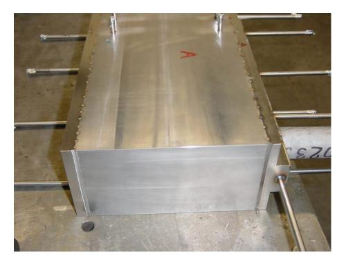
Figure 9: Module during welding. The vertical wall in the foreground of the picture is already welded, the upper walls are fixed.
