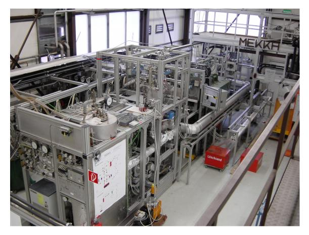
Figure 14: View on the liquid-metal NaK loop in the MEKKA laboratory.
