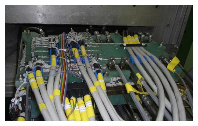
Figure 22: Insulating plates carrying about 600 potential sensors, mounted around the MHD mock-up.
