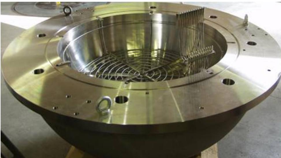
Figure 1: Picture of the LIVE test vessel with volumetric heating system
