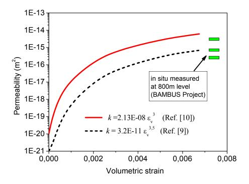
Fig. 2: Permeability of the sample during a transient creep test, calculated using two different relations. For illustration, the permeabilities measured around a large gallery in the Asse mine [9] are plotted.
