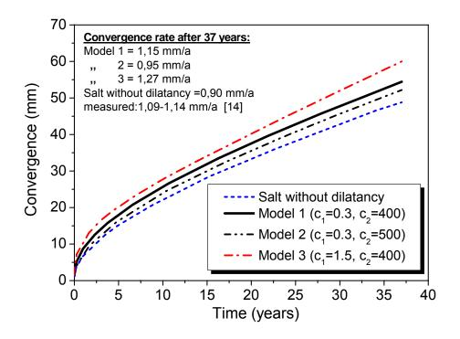
Fig. 9: Gallery convergence calculated for different model parameters and the measured and calculated closure rates 37 years after excavation
