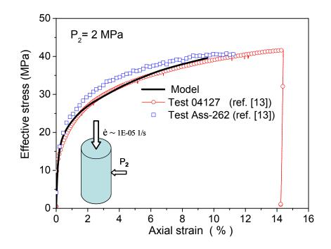
Fig. 6: Comparison of experimental stress-strain curves and calculation
