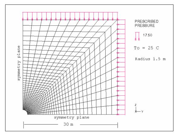
Fig. 8: Finite-element mesh and initial boundary conditions
