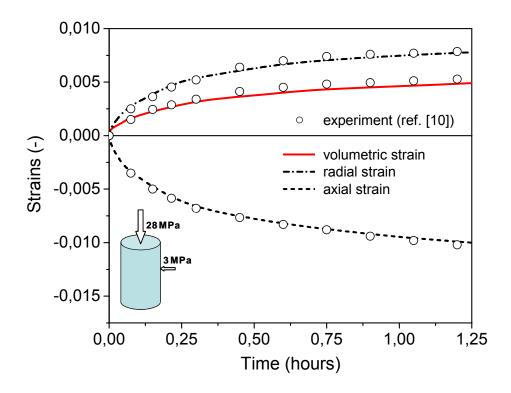
Fig. 1: Comparison between measured creep strains and calculation results
