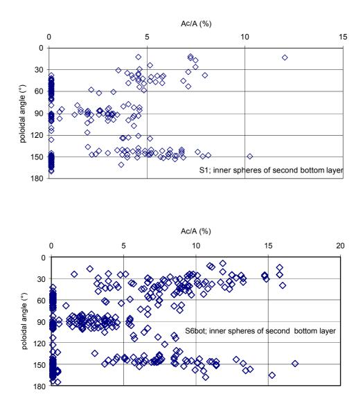
Fig. 4.22. Poloidal distribution of contact surfaces on the inner 2<sup>nd</sup> bottom spheres for samples S1 and S6bot.
