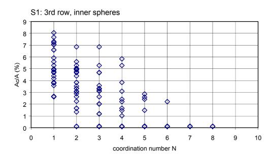
Fig. 4.15. Contact surface distribution on the spheres (sample S1).
