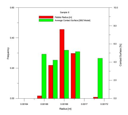
Fig. A.9 – SBZ model contact index by pebble radius size distribution frequency (in green) for sample 6 - middle
