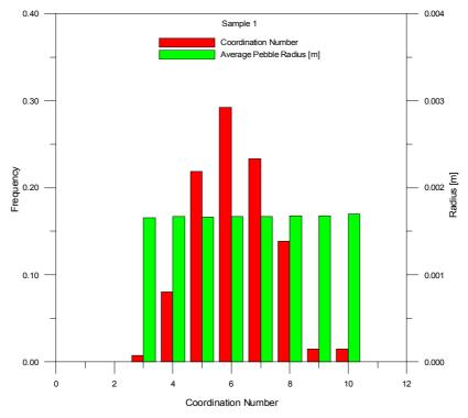
Fig. A.2 – Coordination number (red bars) and pebble average radius (green bars) distribution for sample S1.
