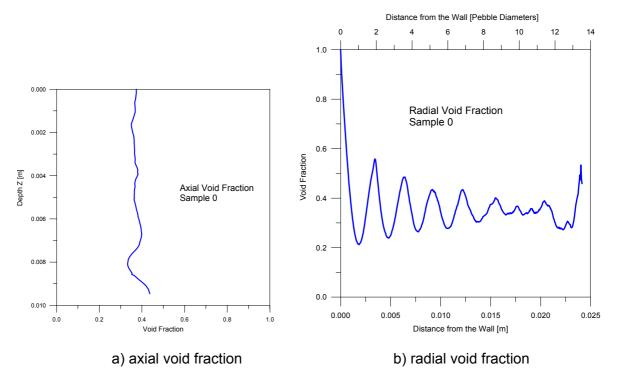
Fig. 3.6. Void fraction profiles for sample S0.
