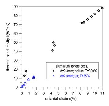
Fig. 2.3 Thermal conductivity as a function of strain for aluminium pebble bed (2mm diameter aluminium spheres).
