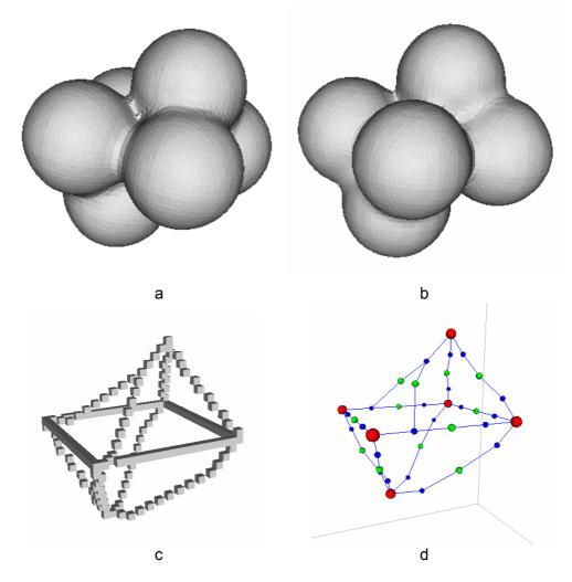
Fig. 4.1. The different steps in the FML Graph extraction: a, b) a six spheres arrangement c) ML skeleton (voxel view) and d) ML graph representation (main nodes in red, connection nodes in green, arcs in blue).
