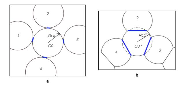
Fig. 4.4. Different pebble configuration cases: a) non-compressed pebbles; and b) compressed pebbles.
