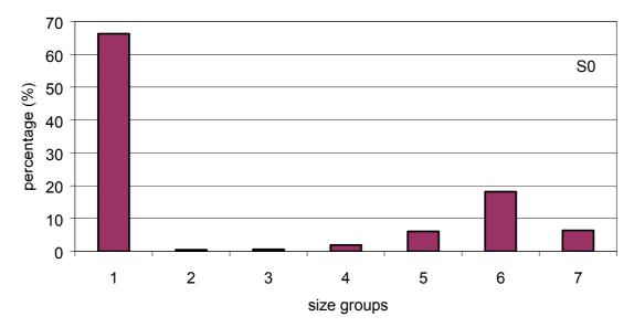
Fig. 4.13. Details of contact surface distribution for S0: (group/Ac/A(%): 1/0.01; 2/(>0.01-0.5); 3(0.5-1.0); 4/(>1.0-1.5); 5/(>1.5-2.0); 6/(>2.0-2.5); 7/(>2.5-3.0).
