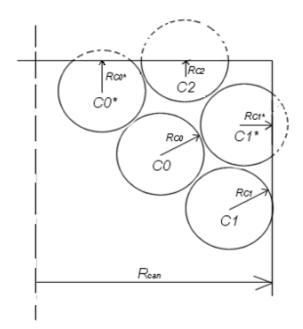
Fig. 4.3. The different classes of pebbles inside a partial domain, representing different radii and coordination numbers.
