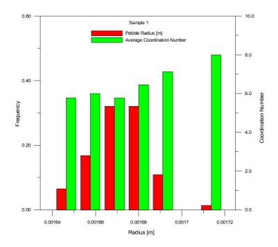
Fig. A.3 – Pebble radius size distribution frequency (red bars) and average coordination number vs. pebble radius (green bars) for sample S1
