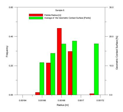
Fig. A.10 – Geometric contact surface index (as defined in Section 4.4)) by pebble radius size distribution frequency for sample 6 - middle
