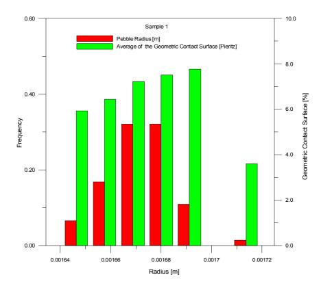
Fig. A.5 – Geometric contact surface index (as defined in section 4.4) by pebble radius size distribution frequency for sample 1
