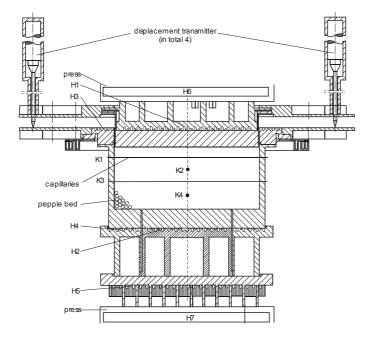
Fig. 1.1. HECOP-facility [2] for measurements of the thermal conductivity of beryllium pebble beds.
