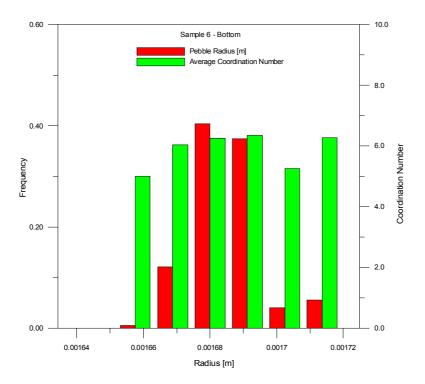
Fig. A.12 – Pebble radius size distribution frequency (red bars) and average coordination number vs. pebble radius (green bars) for sample S6 - bottom
