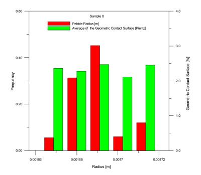
Fig. 4.9. Geometric contact surface index by pebble radius size distribution frequency for sample S0.
