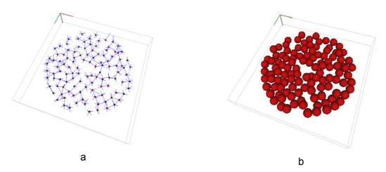
Fig. A.6 – a) ML graph view and b) 3D view of the analysed pebbles (114 objects) of sample S6 - middle
