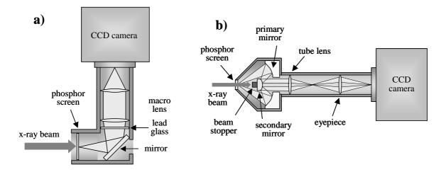
Fig. 2.5 (a) "Low resolution" and (b) "high resolution" imaging detector.
