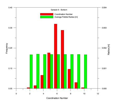
Fig. A.25 – Coordination number (red bars) and pebble average radius (green bars) distribution in sample S6 - bottom
