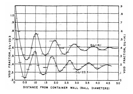
Fig. 3.5. Radial void fraction distribution [18]
