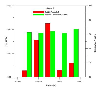
Fig. 4.7. Pebble radius size distribution frequency (red bars) and average coordination number vs. pebble radius (green bars) for sample S0.
