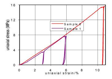
Fig. 2.2 Uniaxial compression tests with pebble beds consisting of 3.5 aluminium spheres.
