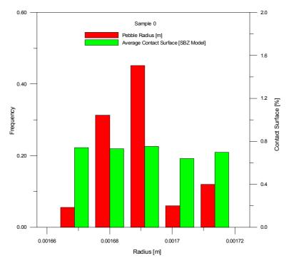
Fig. 4.8. SBZ Contact surface index and pebble radius size distribution frequency (in green) for sample S0.
