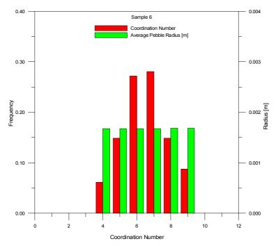
Fig. A.7 – Coordination number (red bars) and pebble average radius (green bars) distribution in sample S6 middle
