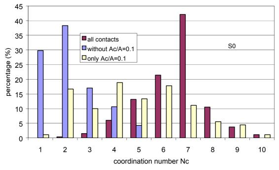
Fig. 4.19. Detailed distribution of coordination numbers for sample S0.
