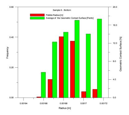
Fig. A.14 – Geometric contact surface index (as defined in section 4.4)) by pebble radius size distribution frequency for sample 6 – bottom.
