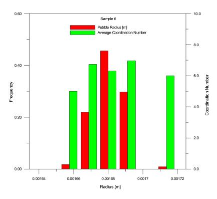
Fig. A.8 – Pebble radius size distribution frequency (red bars) and average coordination number vs. pebble radius (green bars) sample S6 - middle
