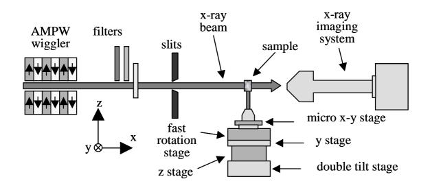
Fig. 2.4 G 4. Schematic view of the x-ray micro-tomography experimental set-up at the ESRF ID15A beam-line. The radiation source is a 7-pole asymmetric wiggler. The x-ray white spectrum is adapted to the different samples by changing the wiggler magnetic field as well as by means of filters.
