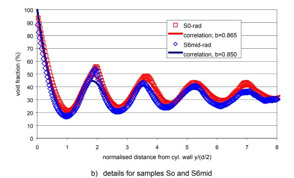
Fig. 3.10. Radial void fraction distributions.
