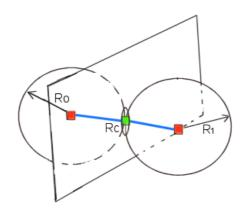
Fig. 4.2. Sphere representation of main nodes with centres R0 and R1 (in red) and connection plane shape with centre Rc (in green) (circular area in the plane).
