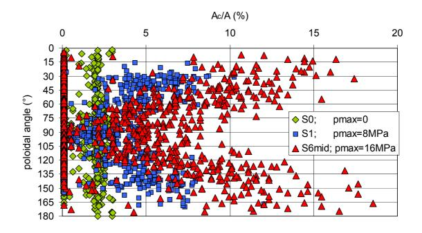
Fig. 4.21. Poloidal distribution of contact surfaces on the spheres.
