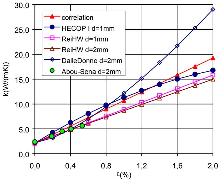
Fig. 5.7. Comparison of Correlation (5.4) with other data ( $T=180^{\circ}\text{C}$ ; except HECOP I:  $T=250^{\circ}\text{C}$ ).
