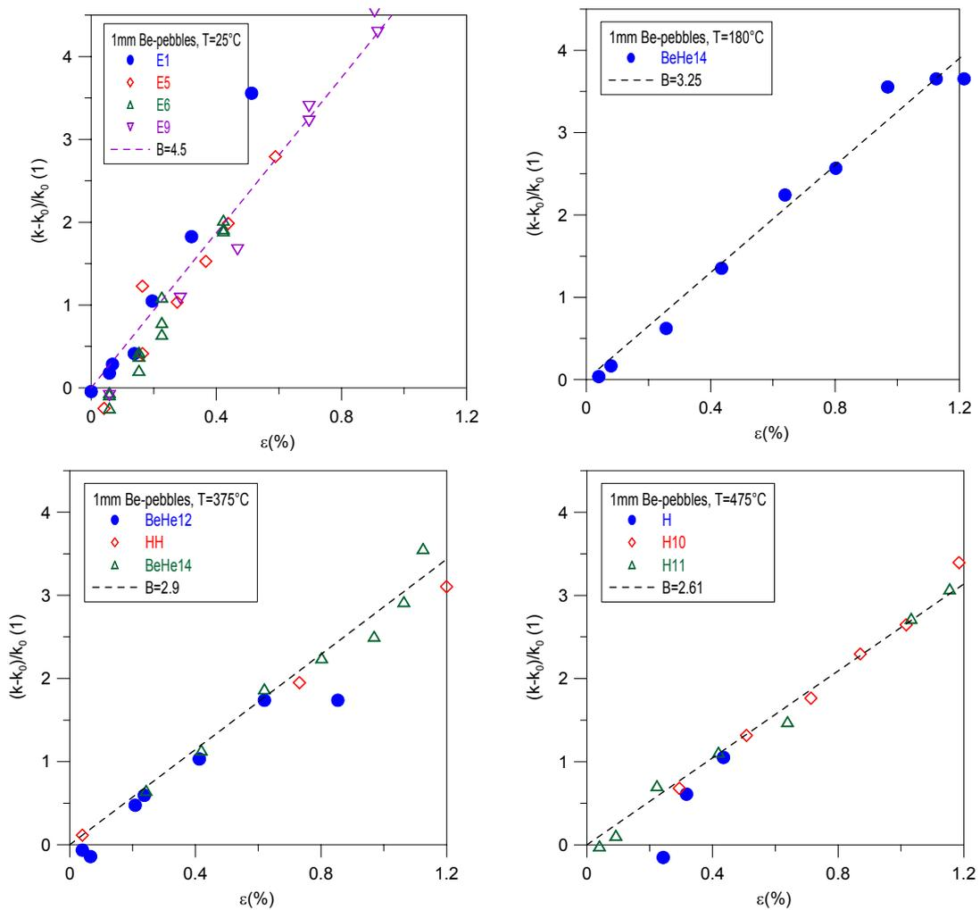
Fig.2.7. Normalised thermal conductivity as a function of strain (1mm pebble beds), ([8])
