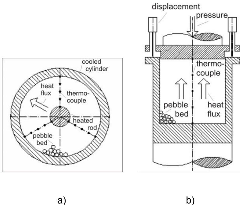
Fig. 1.1. Experimental set-ups used for pebble bed conductivity measurements
