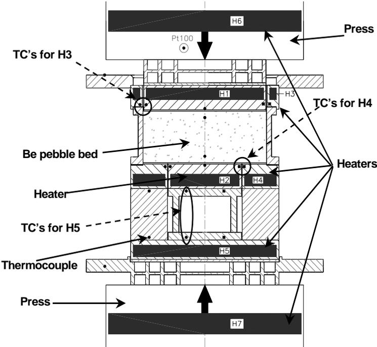
Fig.3.1. HECOP I test section
