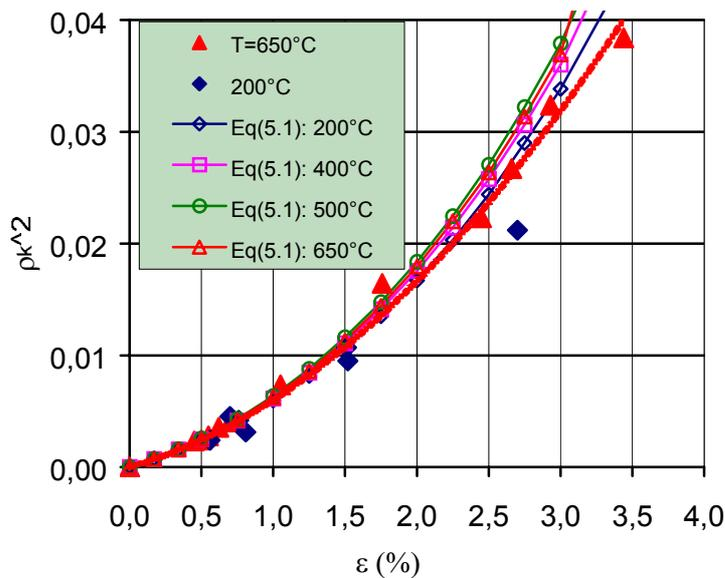
Fig. 5.4. Correlation between  $\rho_k^2$  and measured strains  $\varepsilon$ .
