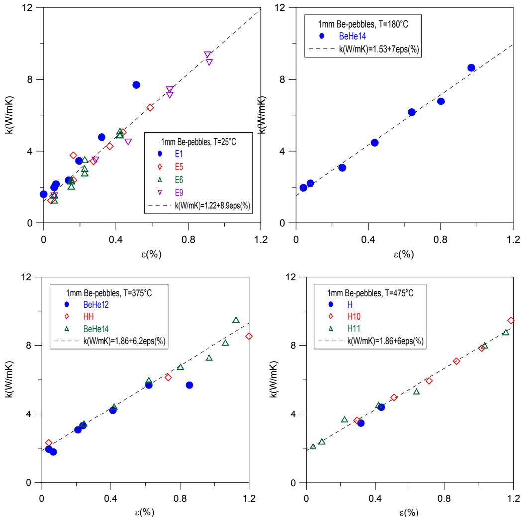
Fig.2.6. Thermal conductivity as a function of strain (1mm pebble beds) ([8]).
