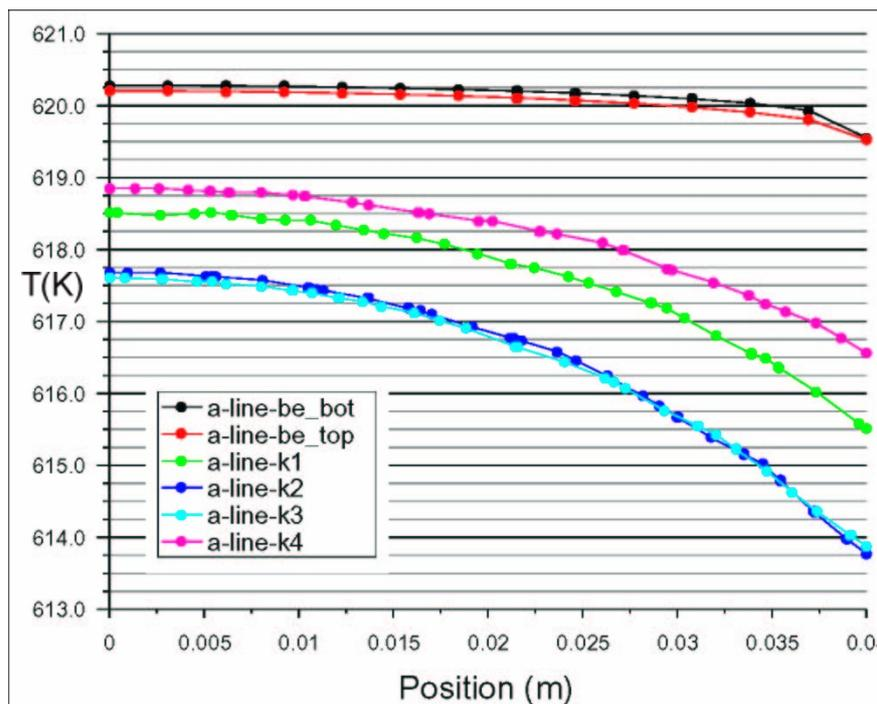
Fig. 3.9. Temperature distribution in pebble bed for  $T_{H2-H4} = T_{H1-H3} = 347^{\circ}\text{C}$ .
