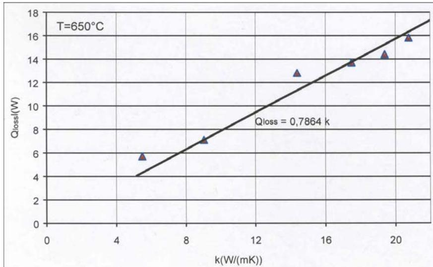
Fig. 4.5. Heat loss correlation for T = 650°C.
