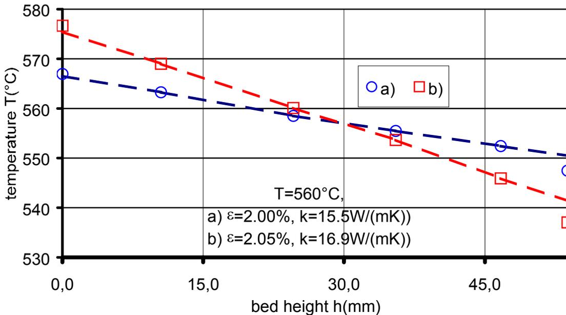
Fig. 4.2. Characteristic axial temperature distributions in the pebble bed.
