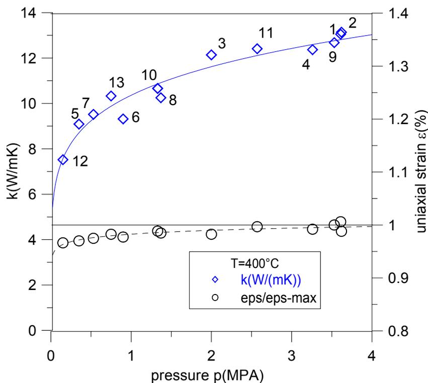
Fig. 4.8. Thermal conductivity during pressure decrease for  $T=400^{\circ}\text{C}$ .
