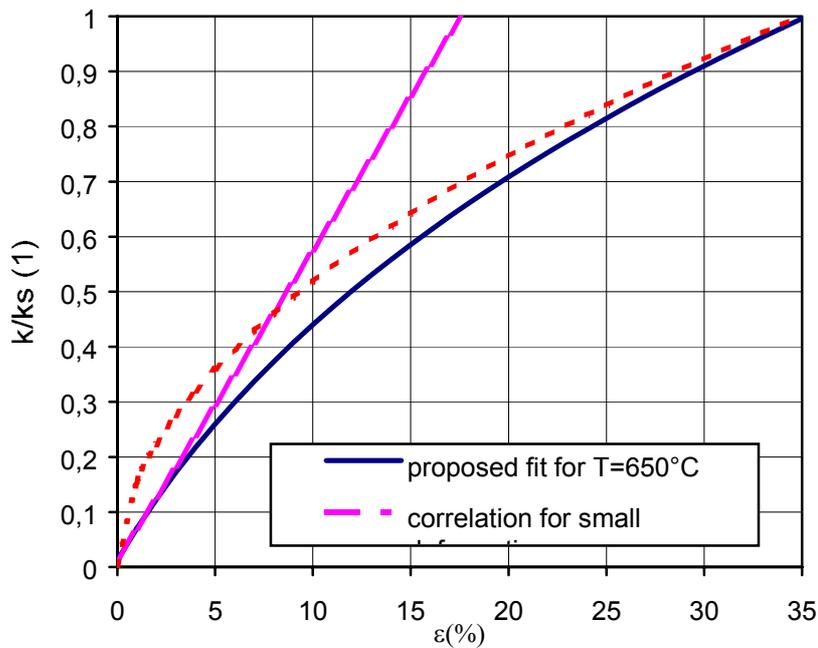
Fig. 5.8. Proposed fit for large bed deformations.
