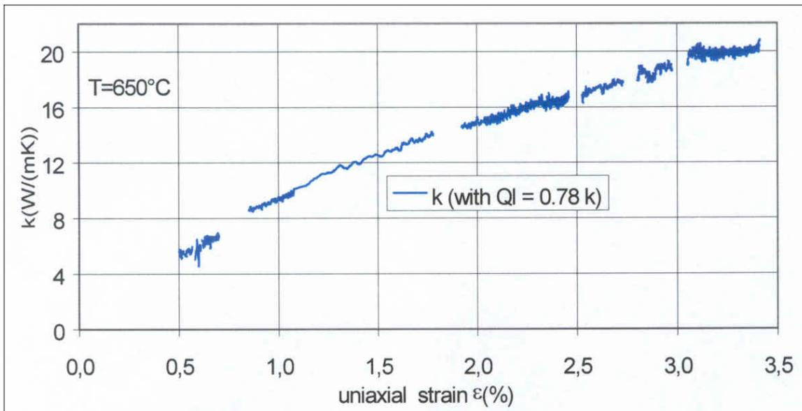
Figure 4.7 Thermal conductivity as a function of strain ( $T = 650^{\circ}\text{C}$ )
