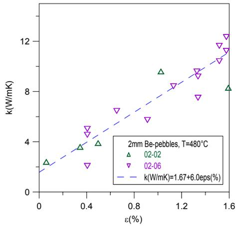
Fig.2.8. Thermal conductivity as a function of strain (2 mm pebble beds), ([8])
