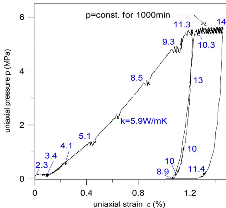
Fig.2.5. Stress-strain dependence for  $T = 485^\circ\text{C}$  and measured conductivities ([8]).
