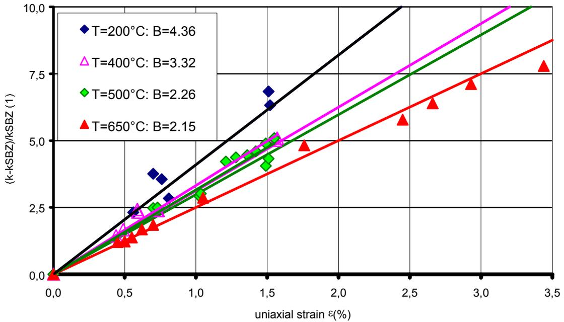
Fig. 5.1. Normalised conductivity as a function of strain.
