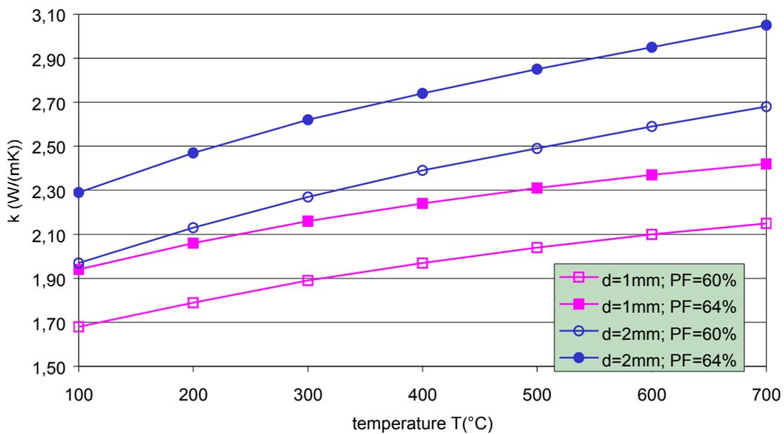
Fig. 2.3. Influence of  $d$  and  $\phi$  for non-deformed beds (SBZ).
