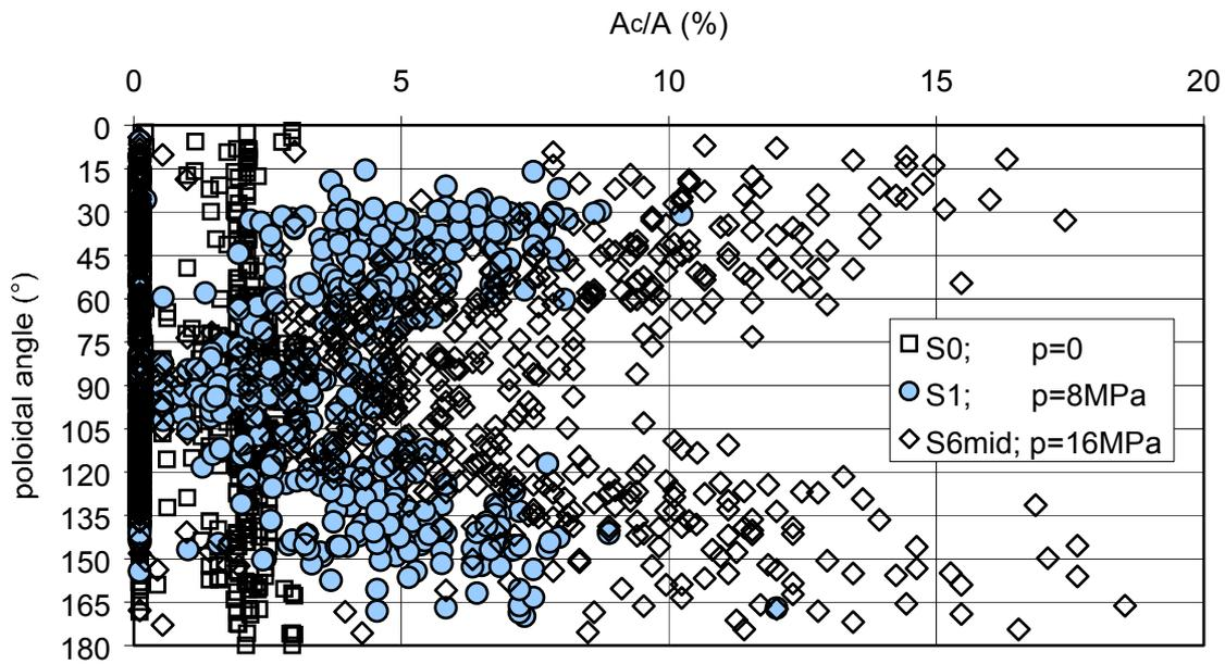
Figure 2.10. Angular distribution of contact surfaces for uniaxially deformed pebble beds (from [15]).
