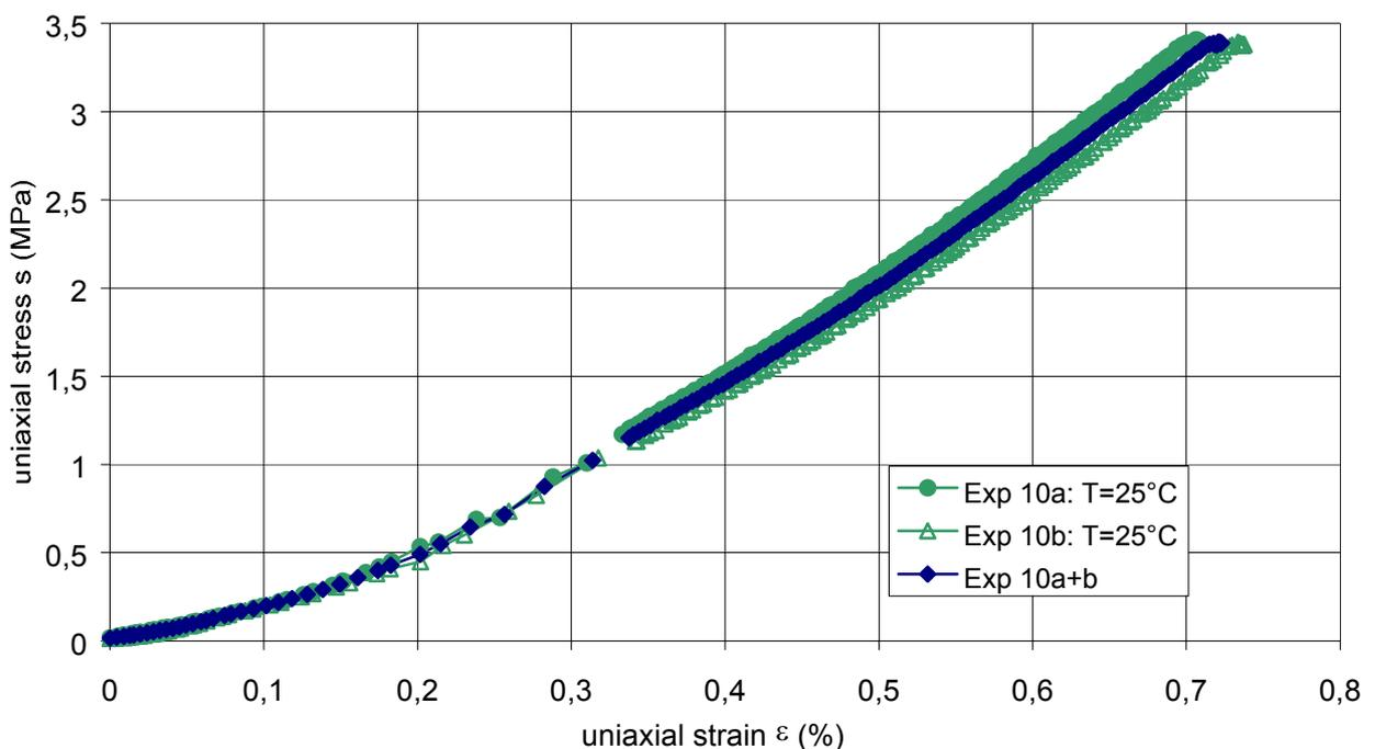
Fig. 4.1. Stress strain relationship for first pressure increase at ambient temperature.
