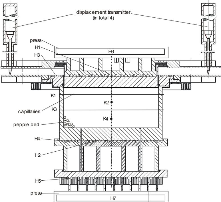
Fig. 3.2. HECOP II test section.
