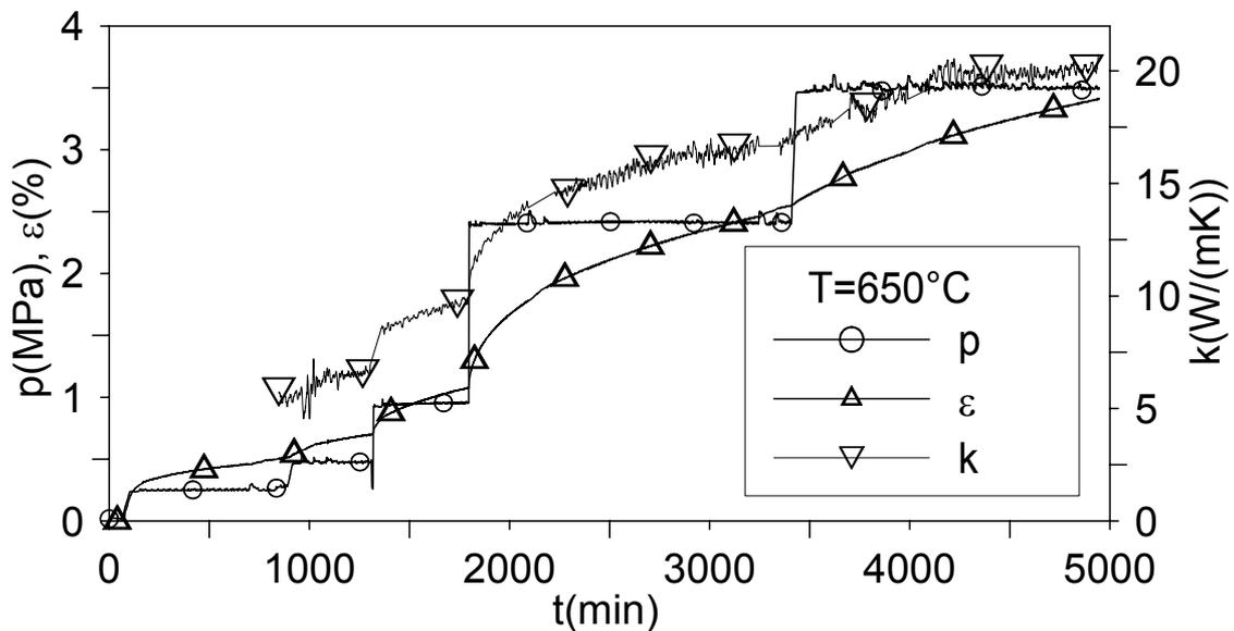
Figure 4.6 Thermal conductivity as a function of time (T = 650°C).
