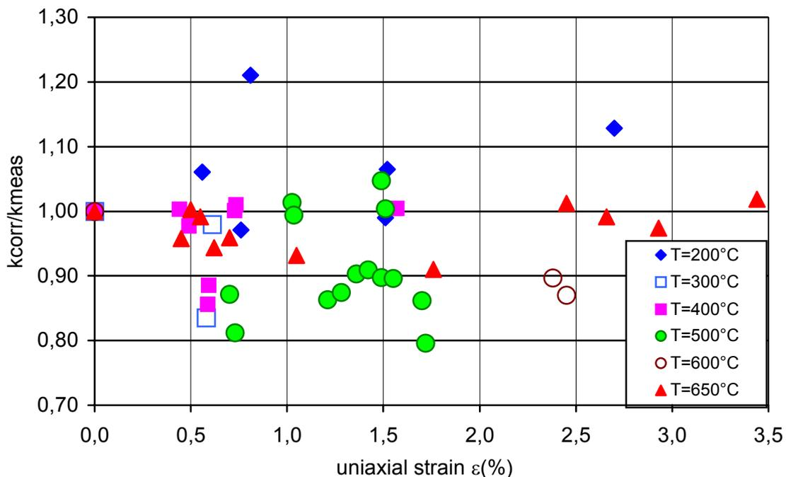
Fig. 5.5. Ratio of  $k_{SBZ}$  using Correlation (5.5) to  $k_{meas}$ .
