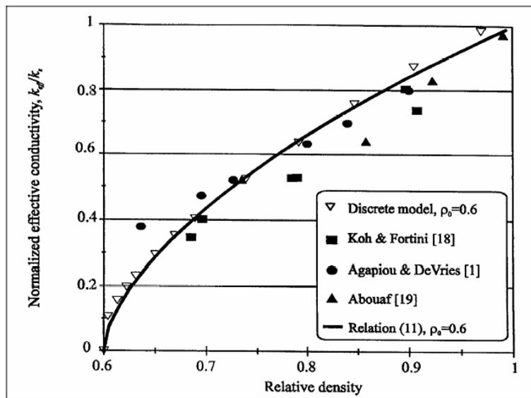
Fig. 2.11 Thermal conductivity of strongly densified pebble beds ([17]).
