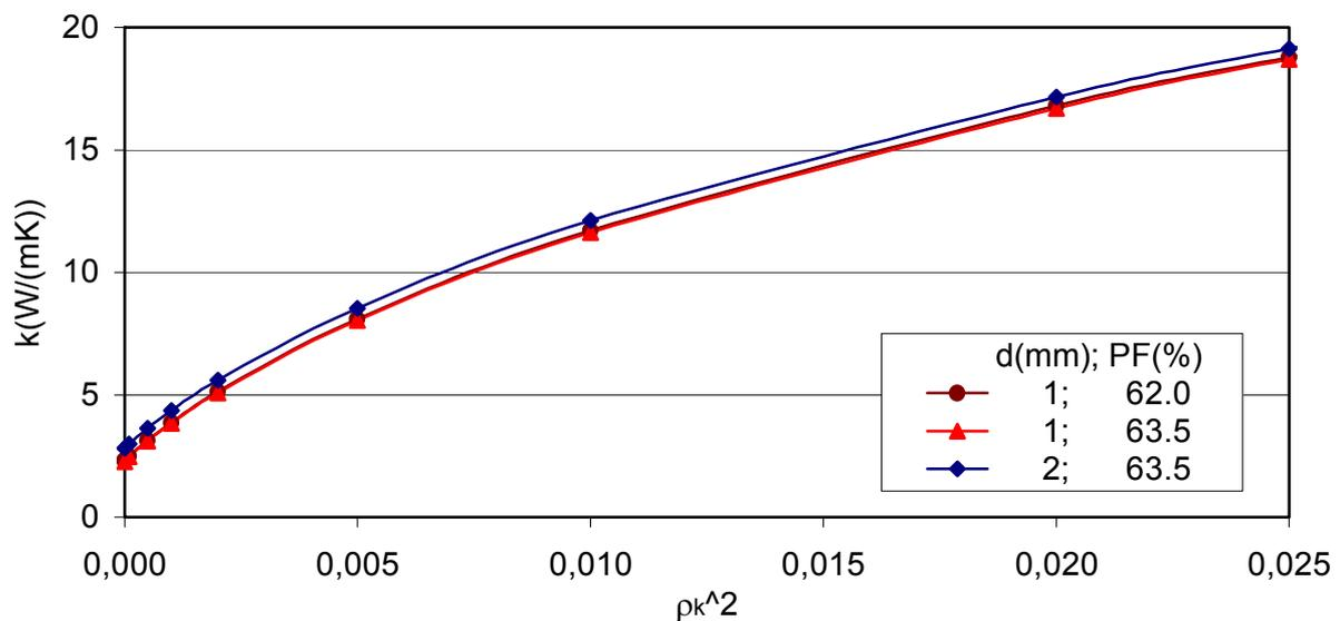
Fig. 5.6 Influence of pebble diameter and packing factor for strongly deformed pebble beds according to SBZ model.
