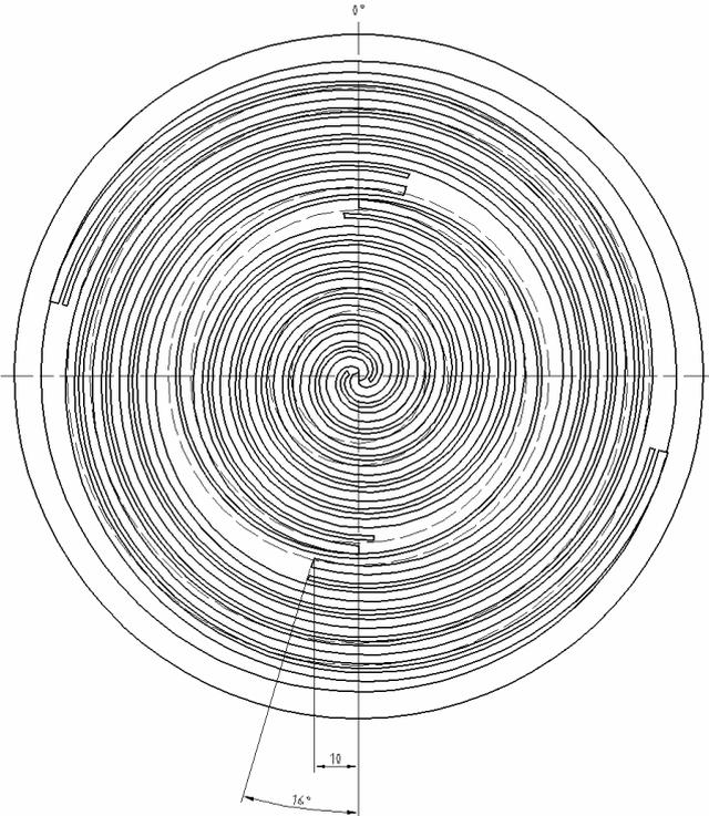
Fig. 3.5. Arrangement of heaters H2 (inner region) and H4 (outer region) in heater plate H2-H4.
