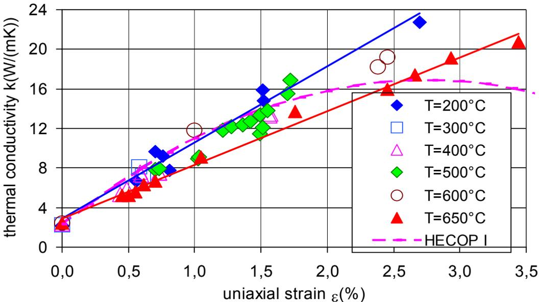
Figure 4.3. Thermal conductivity as a function of strain  $\epsilon$ : all temperatures.
