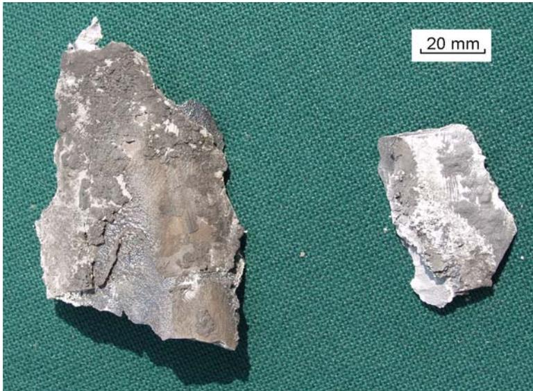
View of the outer shroud surface which was in contact with the  $ZrO_2$  fiber insulation.
