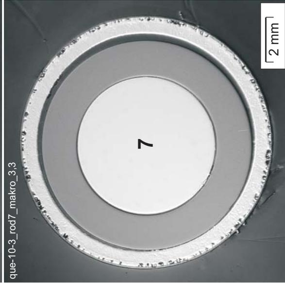
Fig. 73: QUENCH-10; Cross section at 650 mm bundle elevation (QUE-10-3). Macrographs of some rod simulators of the first ring.
