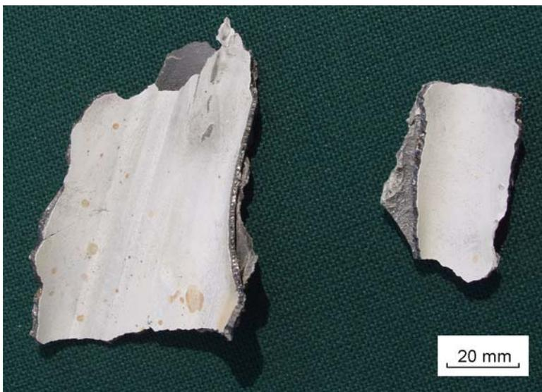
View of the inner side of the shroud. At the fracture surface the  $\alpha$ -Zr(O) metal layer can be recognized. The inner surface is oxidized. There some nitride has formed due to oxidation in air.
