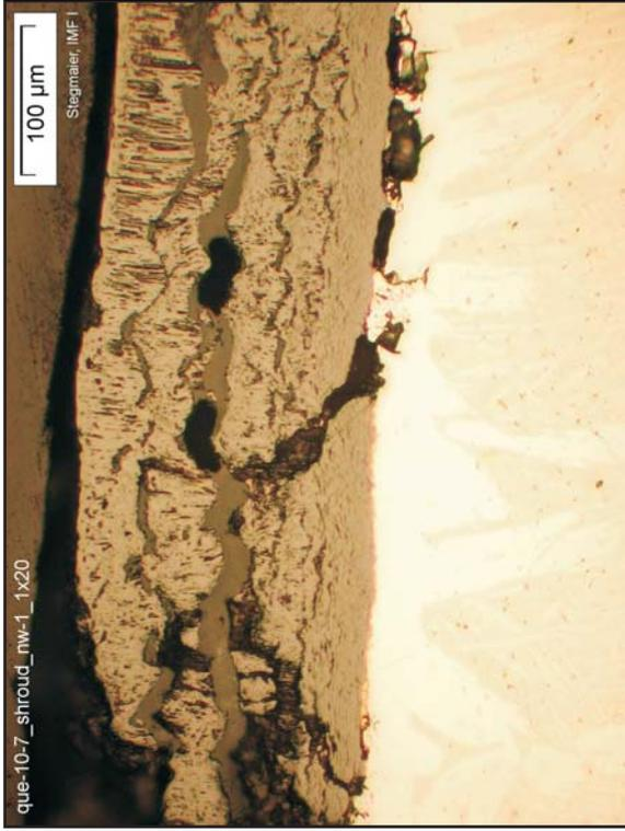
Post-transition scale with lateral cracks
