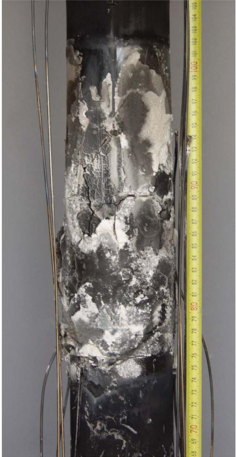
View of the hot zone at  $315^\circ$  orientation of the QUENCH-10 bundle after removal of the  $ZrO_2$  fiber insulation.
