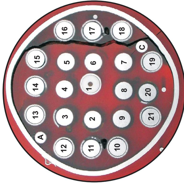
Fig. 102: QUENCH-10; Cross section at 1080 mm bundle elevation (QUE-10-7); overview from top.
