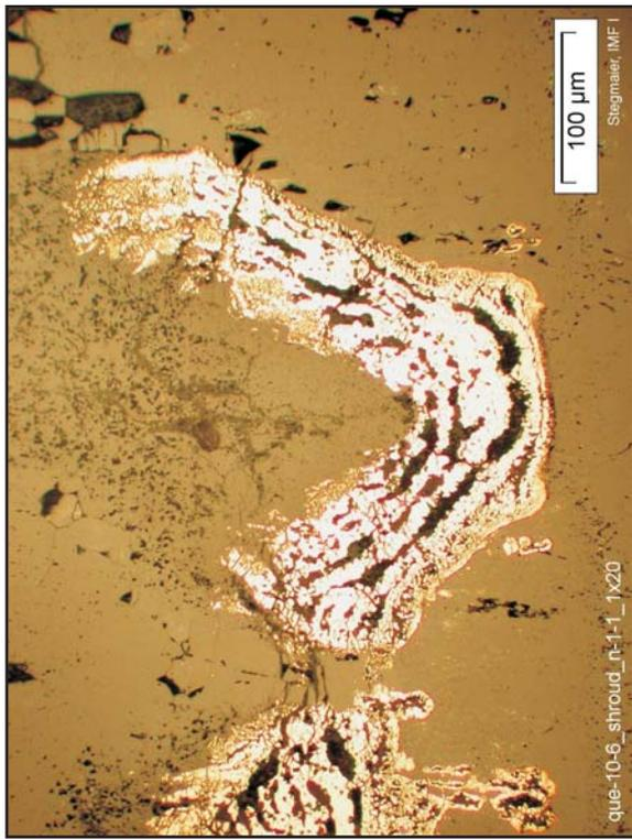
Fig. 100: QUENCH-10; Cross section at 950 mm bundle elevation (QUE-10-6). Shroud towards N, after the air-starved (nitrogen-rich) exposure of the inner scale, and the movement of a re-oxidation front.
