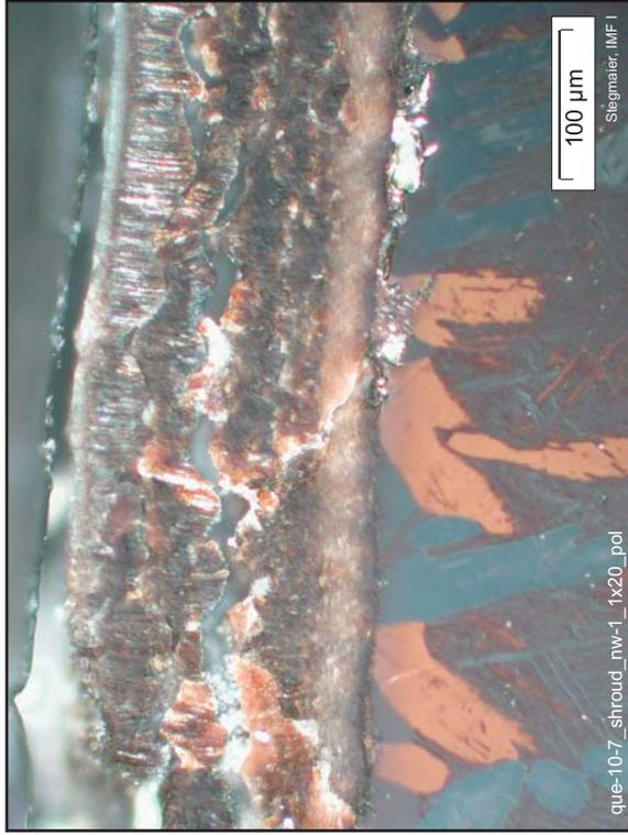
Fig. 108: Cross section at 1080 mm bundle elevation (QUE-10-7). Shroud oxidation, showing the typical pre-transition scale (left), compared to local presence of post-transition scale (right).
