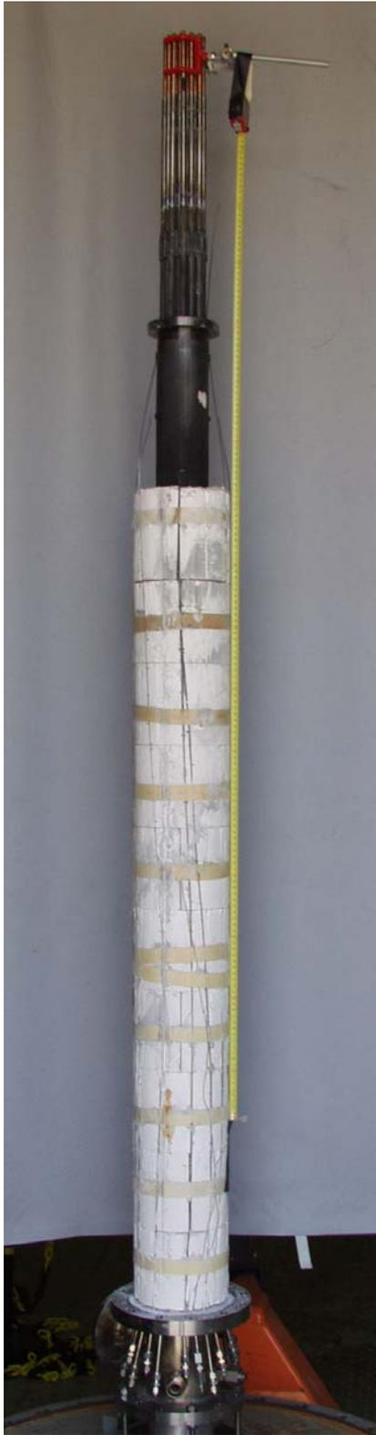
Entire length of the bundle with  $ZrO_2$  fiber insulation at  $315^\circ$  orientation.
