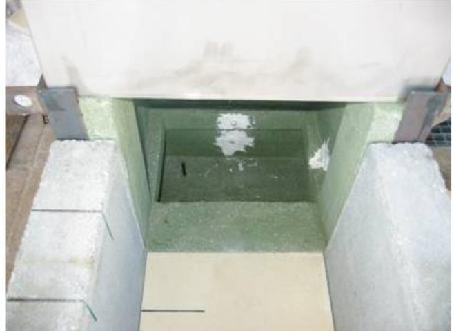
**Figure 2-3:** Thermite reaction vessel and view into the whirl basin in ECOKATS-V1
