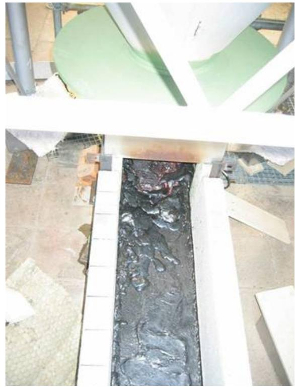
**Figure 2-14:** Spread oxide melt near the whirl basin in ECOKATS-V1
