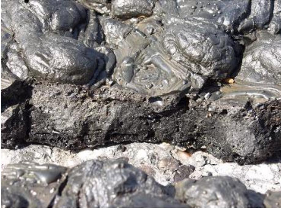
**Figure 3-46:** Cross section of the melt in the middle at  $x = 50$  cm
