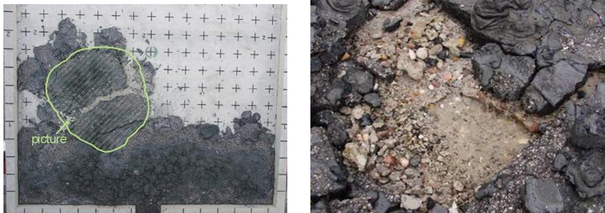
**Figure 3-21:** Area of spalled concrete under the solid melt and detail of the fracture edge
