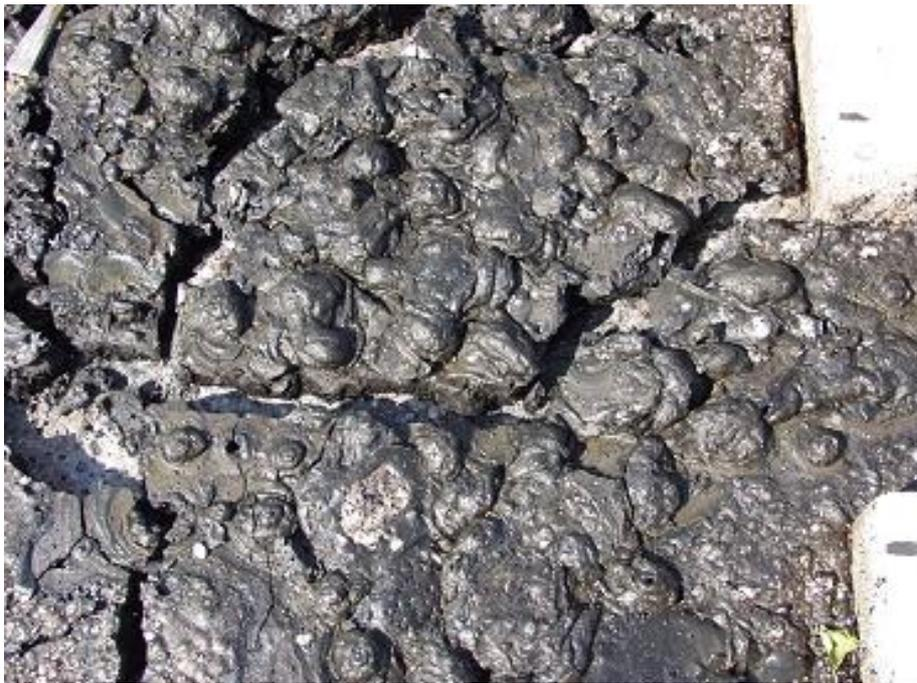
**Figure 3-44:** Profile of the melt in the middle near the supply channel of ECOKATS-1 with fracture lines for the inspection
