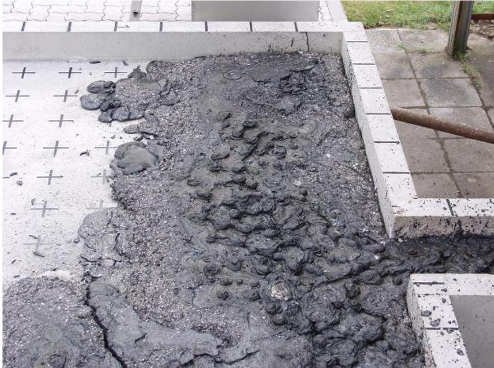
**Figure 3-42:** Right side of the spread melt after cool down
