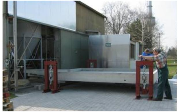
Suspension of the spreading area with load cells
