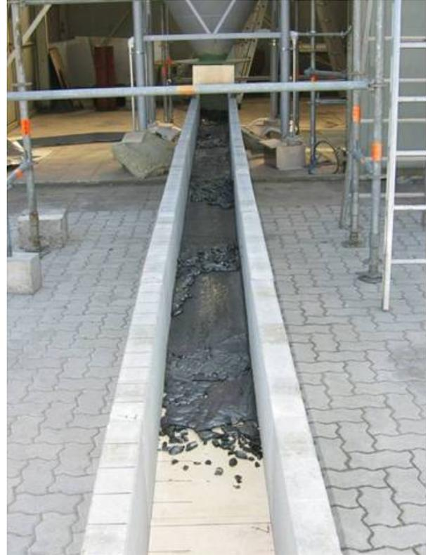
**Figure 2-13:** Total spread oxide melt in ECOKATS-V1
