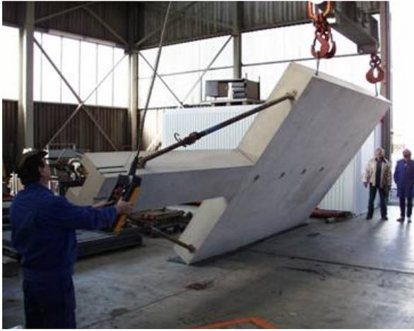
Transport of the large spreading device, view from bottom.
