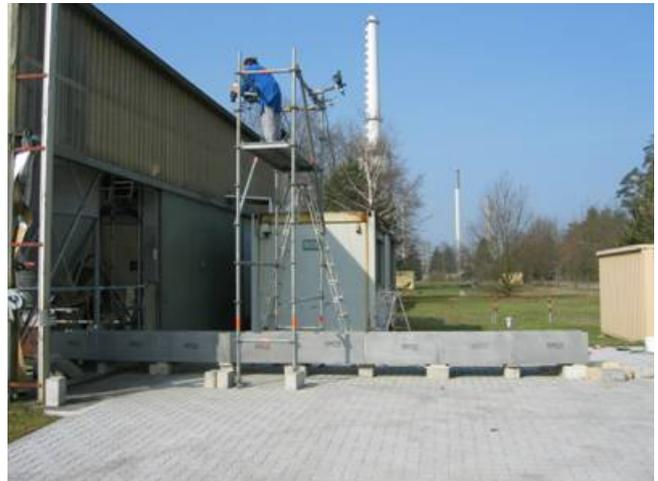
**Figure 2-4:** Front view and side view of the spreading channel of ECOKATS-V1
