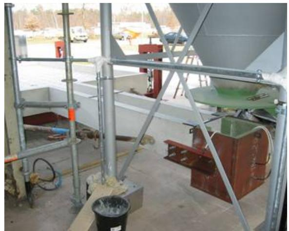
Outlet of thermite vessel, whirl basin, channel and spreading surface
