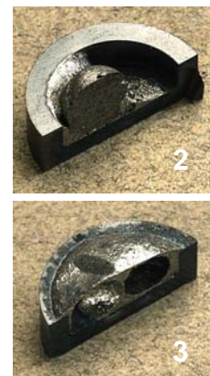
Figure 25: Pre-tests for preparation of absorber melts using powder mixtures. The specimens were either incompletely molten or had large voids.
