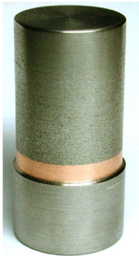
Fig. 5-38: Mo thimble joined through copper layer (option II-A).
