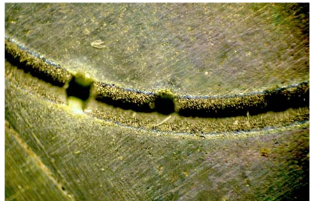
Fig. 5-18: Ring groove (left) and pits (right) on tungsten surface.
