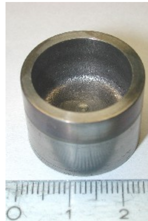
Fig. 5-24: The cup-shaped multi-layer W-V-ferritic steel sample.
