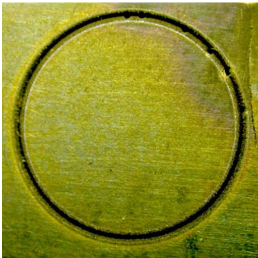
Fig. 5-18: Ring groove (left) and pits (right) on tungsten surface.
