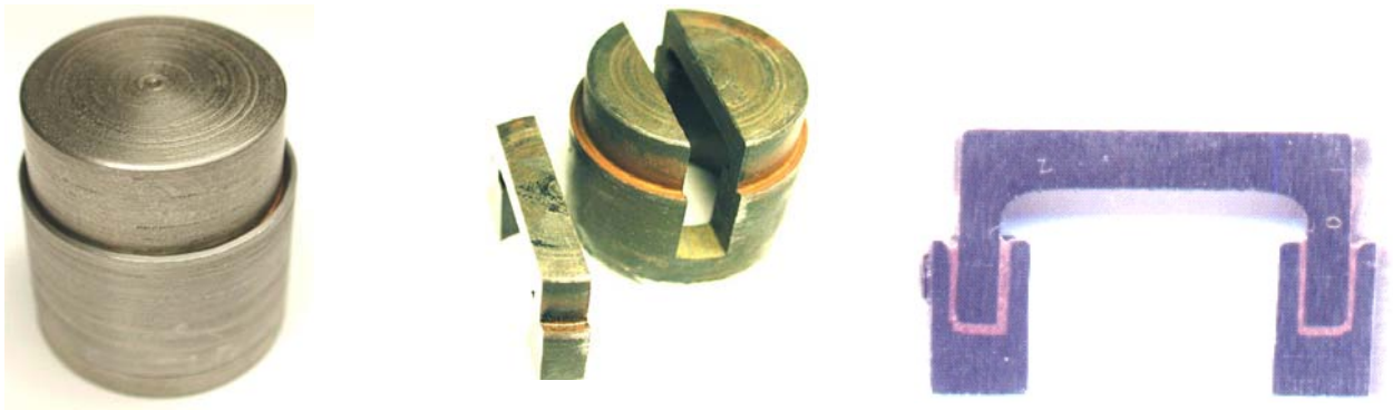
Fig. 5-37: W thimble joined through copper layer (option I-B).
