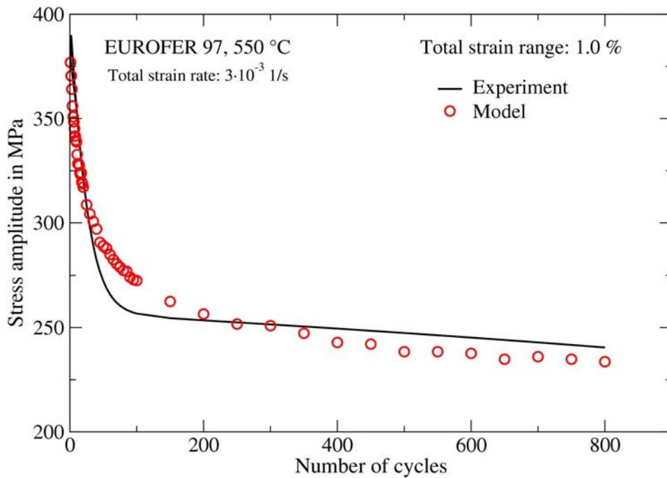
Fig. 4-25 Comparison between material (markers) and model (line) responses for the variation of stress amplitude versus the number of cycles of a strain controlled LCF test
