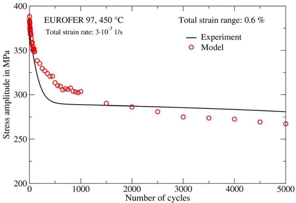
Fig. 4-21 Comparison between material (markers) and model (line) responses for the variation of stress amplitude versus the number of cycles of a strain controlled LCF test
