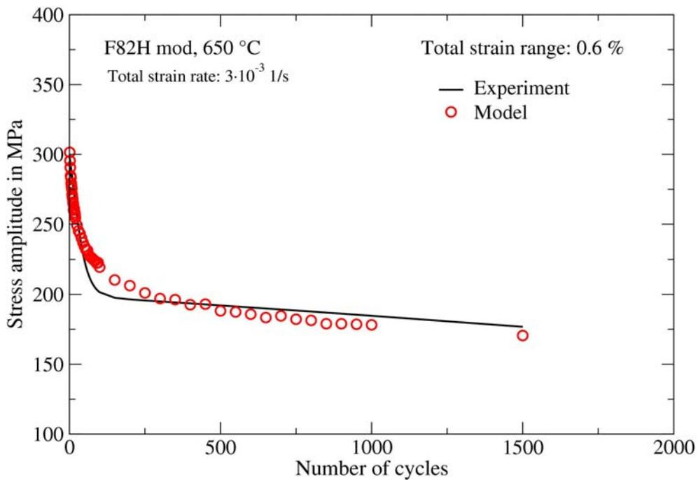
Fig. 4-16 Comparison between material (markers) and model (line) responses for the variation of stress amplitude versus the number of cycles of a strain controlled LCF test
