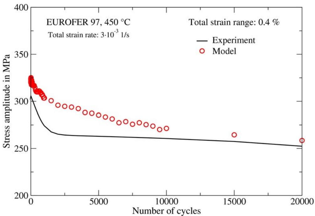
Fig. 4-22 Comparison between material (markers) and model (line) responses for the variation of stress amplitude versus the number of cycles of a strain controlled LCF test
