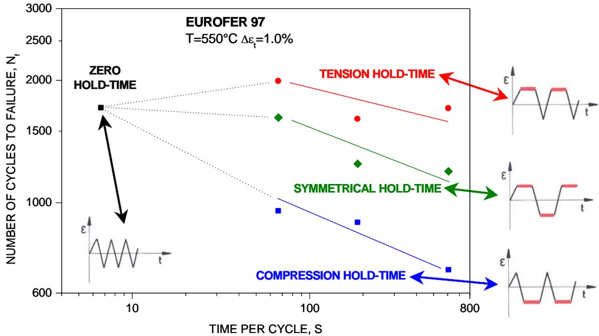
Fig. 2-4 Influence of hold time duration and position on the number of cycles to failure of strain controlled LCF tests
