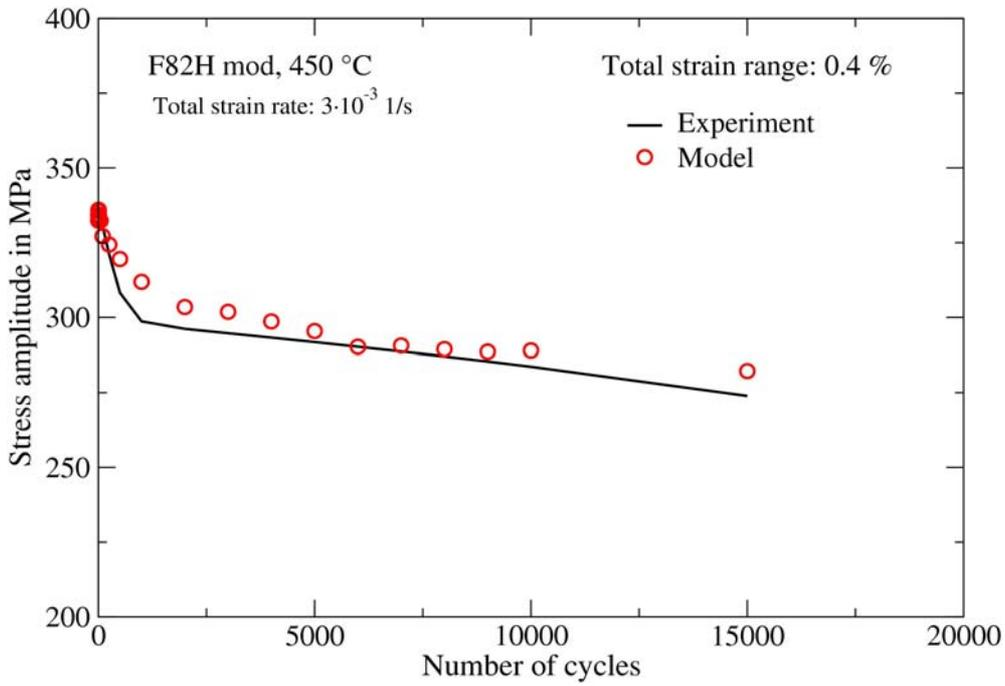
Fig. 4-9 Comparison between material (markers) and model (line) responses for the variation of stress amplitude versus the number of cycles of a strain controlled LCF test
