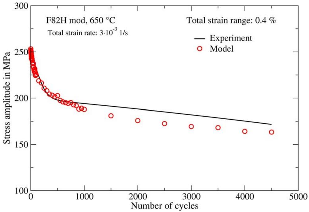
Fig. 4-17 Comparison between material (markers) and model (line) responses for the variation of stress amplitude versus the number of cycles of a strain controlled LCF test
