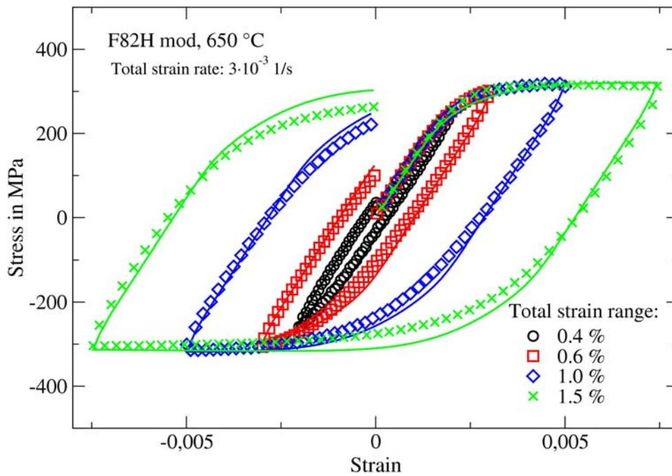
Fig. 4-13 Comparison between material (markers) and model (line) responses for the first stress strain hysteresis of strain controlled LCF tests performed with different total strain ranges
