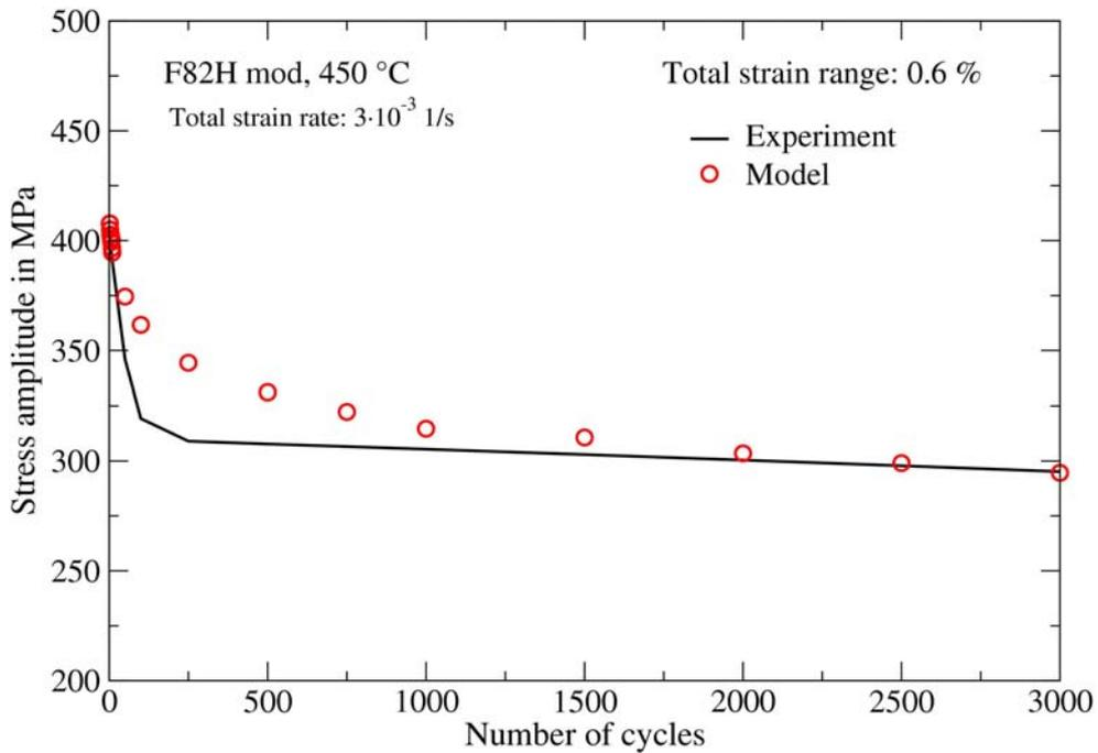
Fig. 4-8 Comparison between material (markers) and model (line) responses for the variation of stress amplitude versus the number of cycles of a strain controlled LCF test
