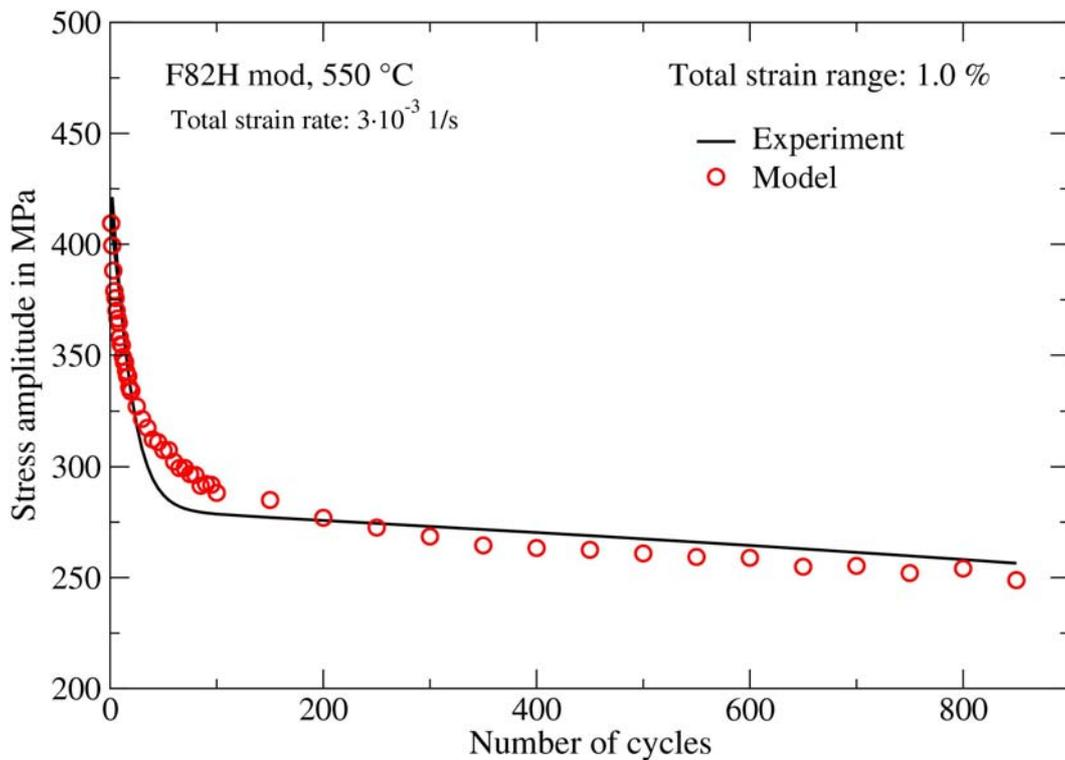
Fig. 4-2 Comparison between material (markers) and model (line) responses for the variation of stress amplitude versus the number of cycles of a strain controlled LCF test
