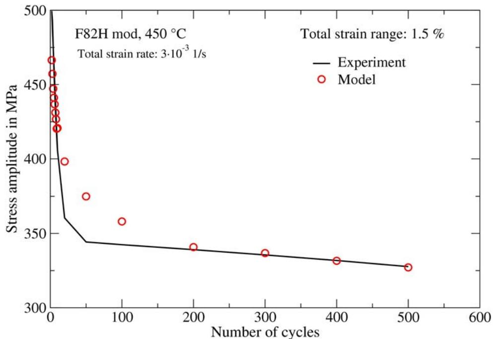
Fig. 4-6 Comparison between material (markers) and model (line) responses for the variation of stress amplitude versus the number of cycles of a strain controlled LCF test
