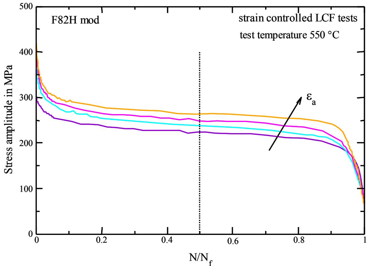
Fig. 2-1 Stress amplitude versus normalized number of cycles for strain controlled LCF tests with different strain amplitudes
