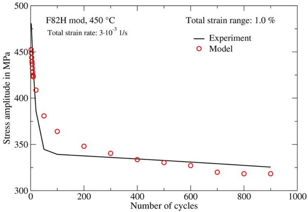
Fig. 4-7 Comparison between material (markers) and model (line) responses for the variation of stress amplitude versus the number of cycles of a strain controlled LCF test
