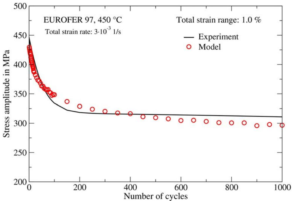
Fig. 4-20 Comparison between material (markers) and model (line) responses for the variation of stress amplitude versus the number of cycles of a strain controlled LCF test
