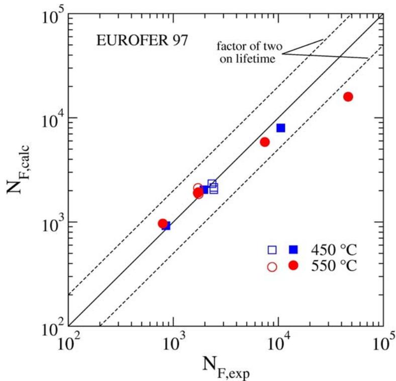
Fig. 4-4 Comparison between numbers of cycles to failure calculated by the coupled deformation damage model with those determined experimentally for EUROFER97 in LCF tests without (solid symbols) and with hold time (open symbols)
