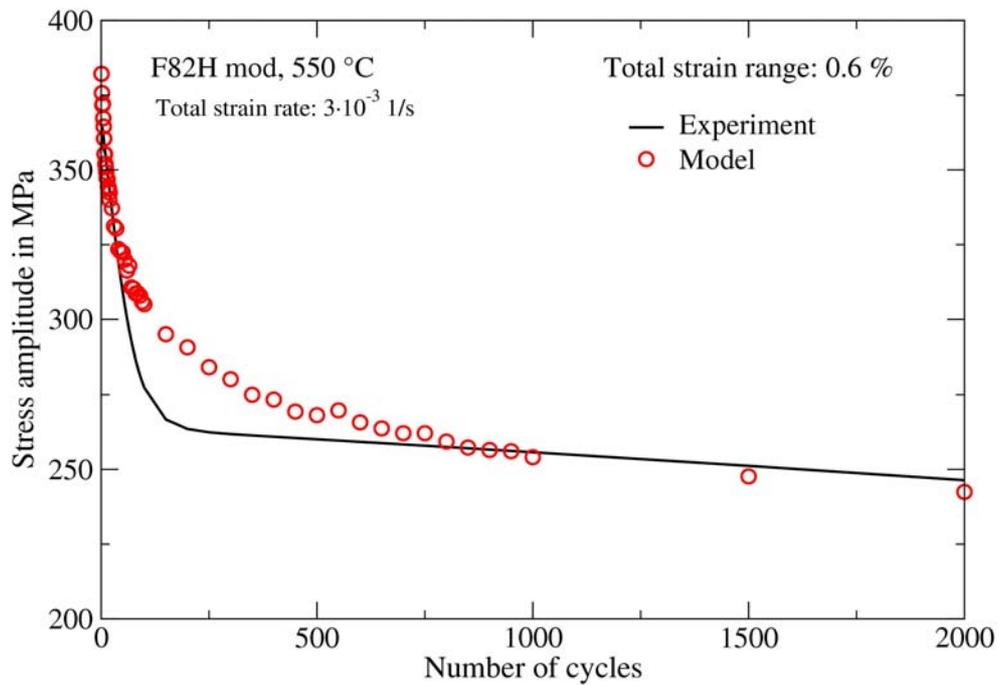
Fig. 4-11 Comparison between material (markers) and model (line) responses for the variation of stress amplitude versus the number of cycles of a strain controlled LCF test
